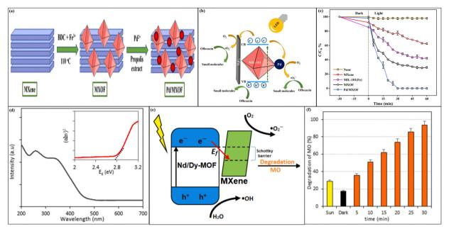
Fig. 5 (a) Synthesis of the Pd/MXOF nanocomposite, (b) degradation of ofloxacin (OFL), and (c) percent degradation of MXene, MOF, MXOF, and Pd/ MXOF. Reproduced with permission from ref. 59. Copyright 2024, Elsevier. (d) Bandgap of Nd/Dy-MOF@MXene, (e) mechanism of methyl orange (MO) degradation, and (f) degradation of MO vs. time. Reproduced with permission from ref. 84. Copyright 2025, Elsevier.
