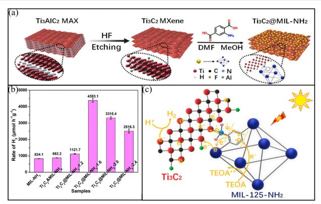
Fig. 12 (a) Schematic preparation process of  $Ti_3C_2@MIL-NH_2$ , (b)  $H_2$  production over the  $MIL-NH_2$ ,  $Ti_3C_2@MIL-NH_2$  and  $Ti_3C_2@MIL-NH_2$  composites, and (c) mechanism for  $H_2$  production over the  $Ti_3C_2@MIL-NH_2$  composite. Reproduced with permission from ref. 104. Copyright 2021, Elsevier.
