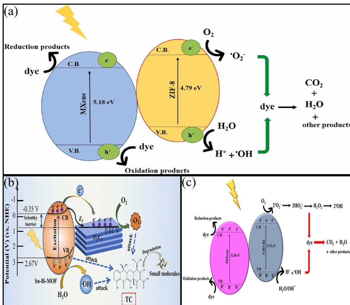
Fig. 11 (a) The degradation method by the MXOF nanocomposite. Reproduced with permission from ref. 69. Copyright 2023, Elsevier. (b) The suggested photocatalytic mechanism in  $\text{Sn-Bi-MOF}/\text{Ti}_3\text{C}_2$ .<sup>87</sup> (c) Schematic representation of MB and DR31 degradation mechanism using  $\text{MXene}@/\text{UiO-66}$  nanocomposite. Reproduced with permission from ref. 68. Copyright 2024, Elsevier.
