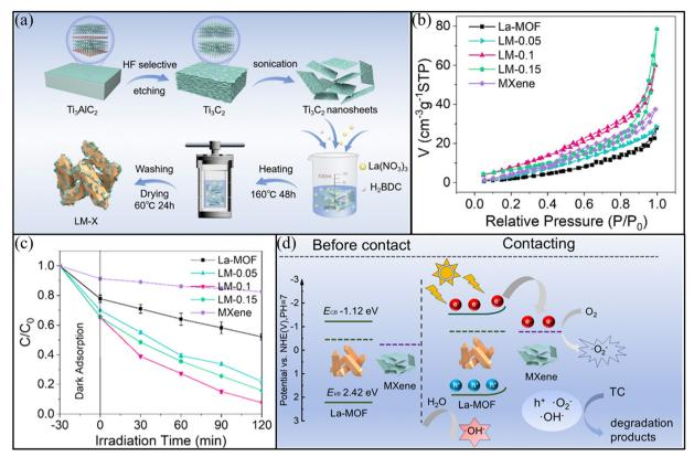
Fig. 7 (a) Schematic representation of the preparation of LM-0.1, (b) N<sub>2</sub> adsorption-desorption isotherms, (c) TC removal with a xenon lamp and (d) possible method for degradation of TC by LM-0.1 under solar light exposure. Reproduced with permission from ref. 85. Copyright 2025, Elsevier.
