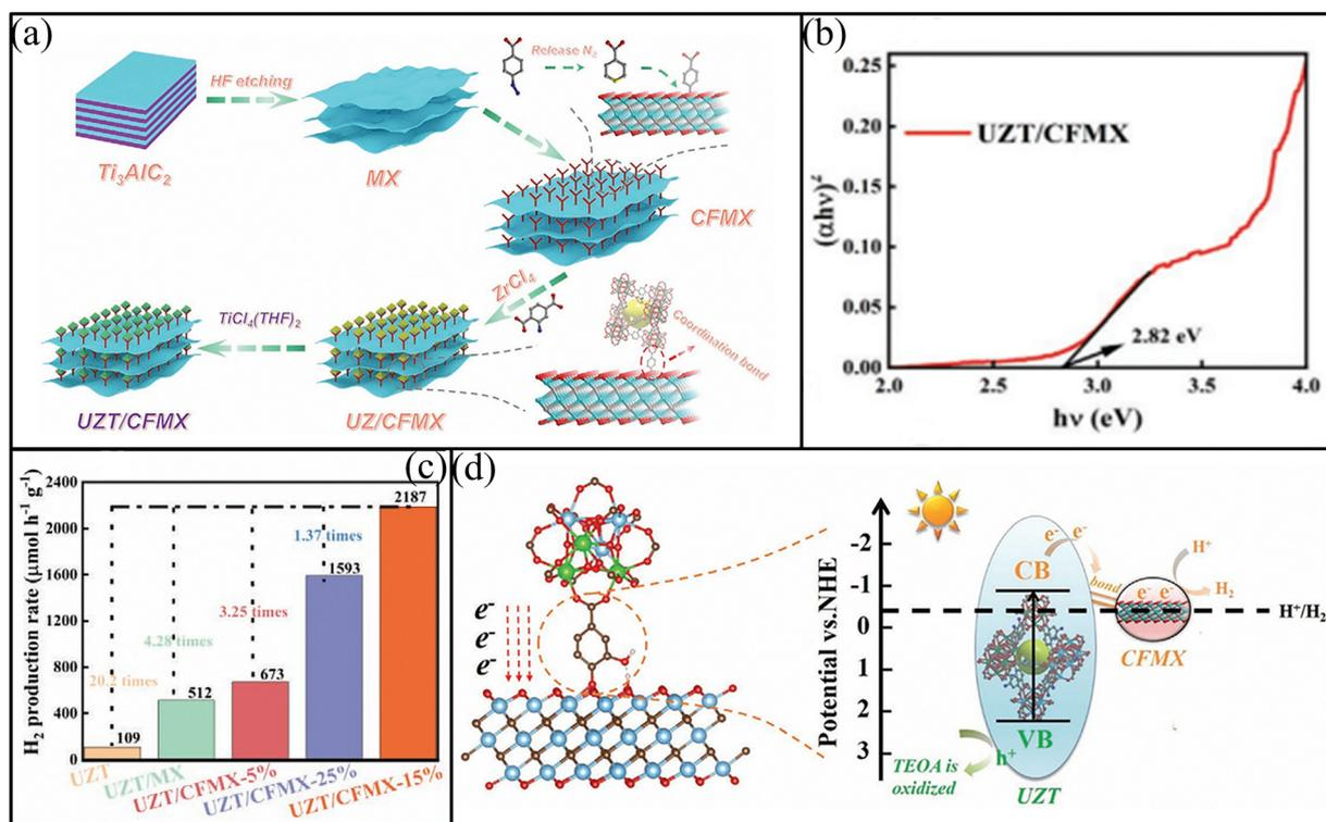
Fig. 13 (a) Schematic illustration of the construction of the UZT/CFMX heterostructure, (b) bandgap of UZT/CFMX, (c) H<sub>2</sub> production of UZT, UZT/MX, UZT/CFMX-5%, UZT/CFMX-15%, and UZT/CFMX-25%, and (d) photocatalytic water splitting mechanism for UZT/CFMX. Reproduced with permission from ref. 101. Copyright 2022, open access CC BY 4.0.
