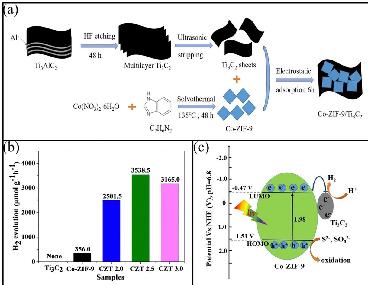
Fig. 14 (a) Synthesis of Co-ZIF-9/Ti<sub>3</sub>C<sub>2</sub>, (b) comparison of the H<sub>2</sub>-production rate over different samples, and (c) mechanism for H<sub>2</sub>-evolution over the Co-ZIF-9/Ti<sub>3</sub>C<sub>2</sub>. Reproduced with permission from ref. 105. Copyright 2022.
