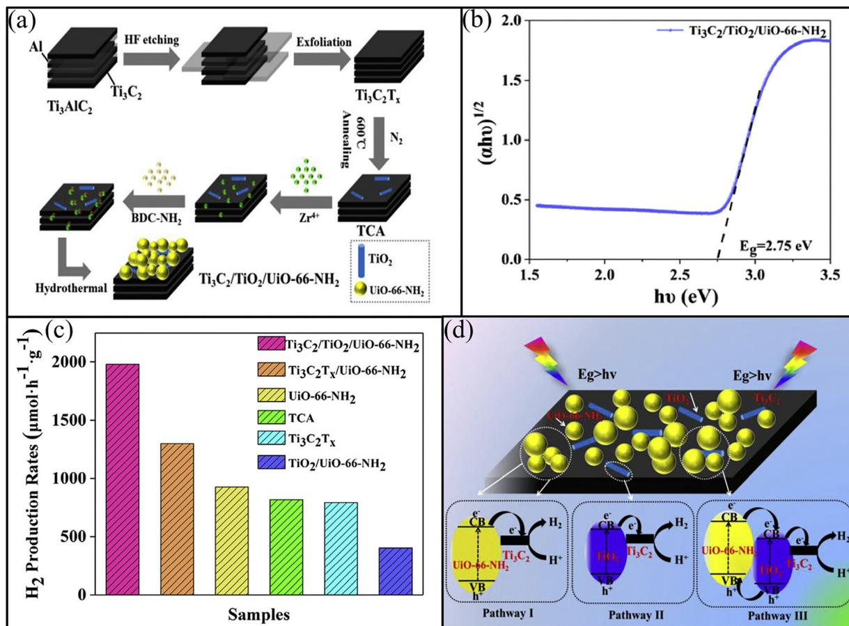
Fig. 15 (a) Diagrammatic representation of a possible chemical route for the synthesis of  $\text{Ti}_3\text{C}_2/\text{TiO}_2/\text{UiO-66-NH}_2$ , (b) bandgap for the  $\text{Ti}_3\text{C}_2/\text{TiO}_2/\text{UiO-66-NH}_2$  nanocomposite, (c) the as-prepared samples had average  $\text{H}_2$  production, and (d) the charge-transfer paths for  $\text{Ti}_3\text{C}_2/\text{TiO}_2/\text{UiO-66-NH}_2$  are shown schematically. Reproduced with permission from ref. 52. Copyright 2019, Elsevier.
