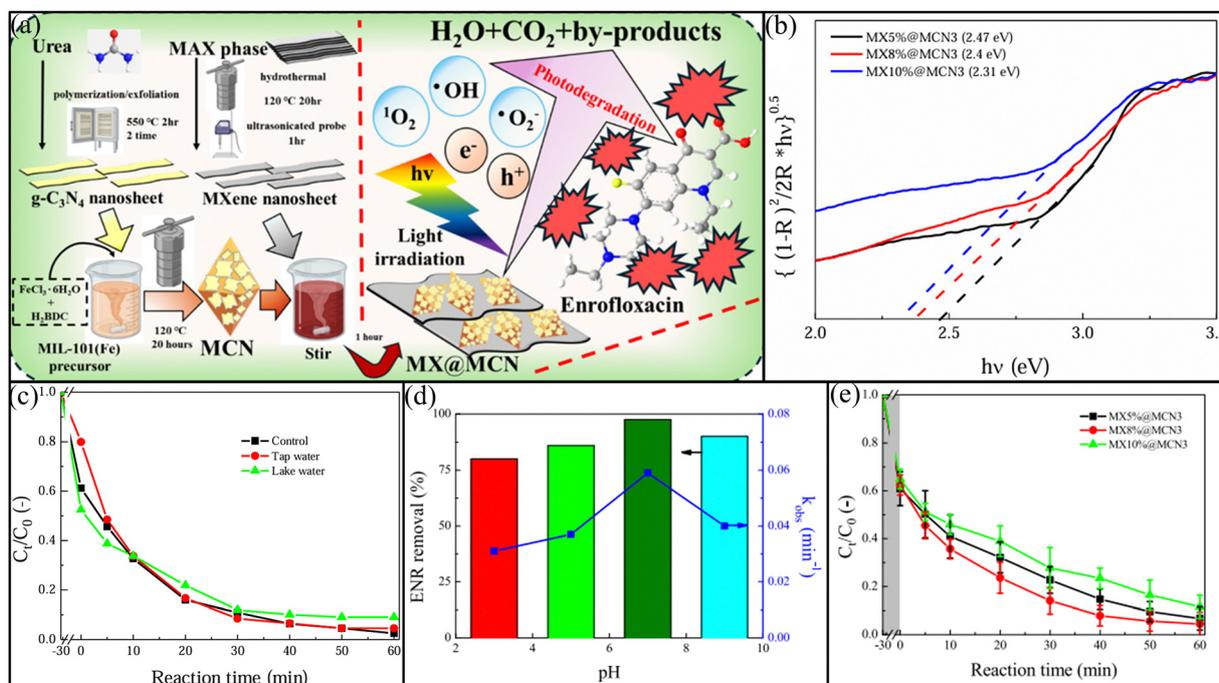
Fig. 6 (a) Synthesis of MX@MCN and its photocatalytic activity against enrofloxacin degradation through light, (b) bandgap of the MX@MCN nanocomposite, (c) impact of the water matrix on the photodegradation of ENR over the MX@MCN photocatalyst when exposed to visible light, (d) pH study of MX@MCN, and (e) photodegradation of enrofloxacin (ENR) over MX@MCN. Reproduced with permission from ref. 58. Copyright 2025, Elsevier.
