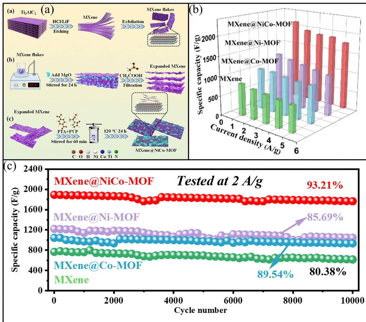
Fig. 17 (a) A simplified representation of the fabrication method of the MXene@NiCo-MOF, (b) specific capacitance of four electrodes, and (c) cycling stability for 10 000 cycles of the as-prepared electrode. Reproduced with permission from ref. 114. Copyright 2024, Elsevier.
