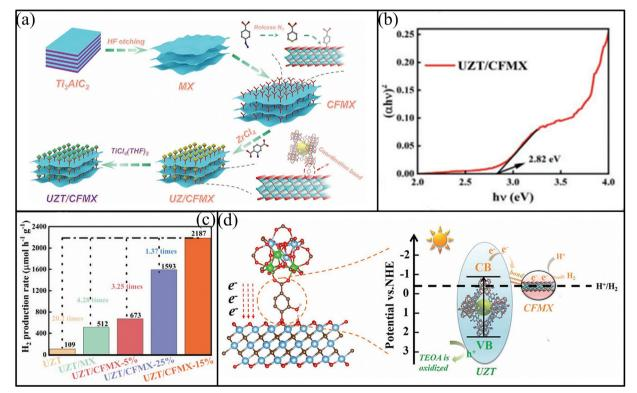
Fig. 13 (a) Schematic illustration of the Construction of the UZT/CFMX heterostructure, (b) bandgap of UZT/CFMX, (c)  $H_2$  production of UZT, UZT/MX, UZT/CFMX-5%, UZT/CFMX-15%, and UZT/CFMX-25%, and (d) photocatalytic water splitting mechanism for UZT/CFMX. Reproduced with permission from ref. 101. Copyright 2022, open access CC BY 4.0.
