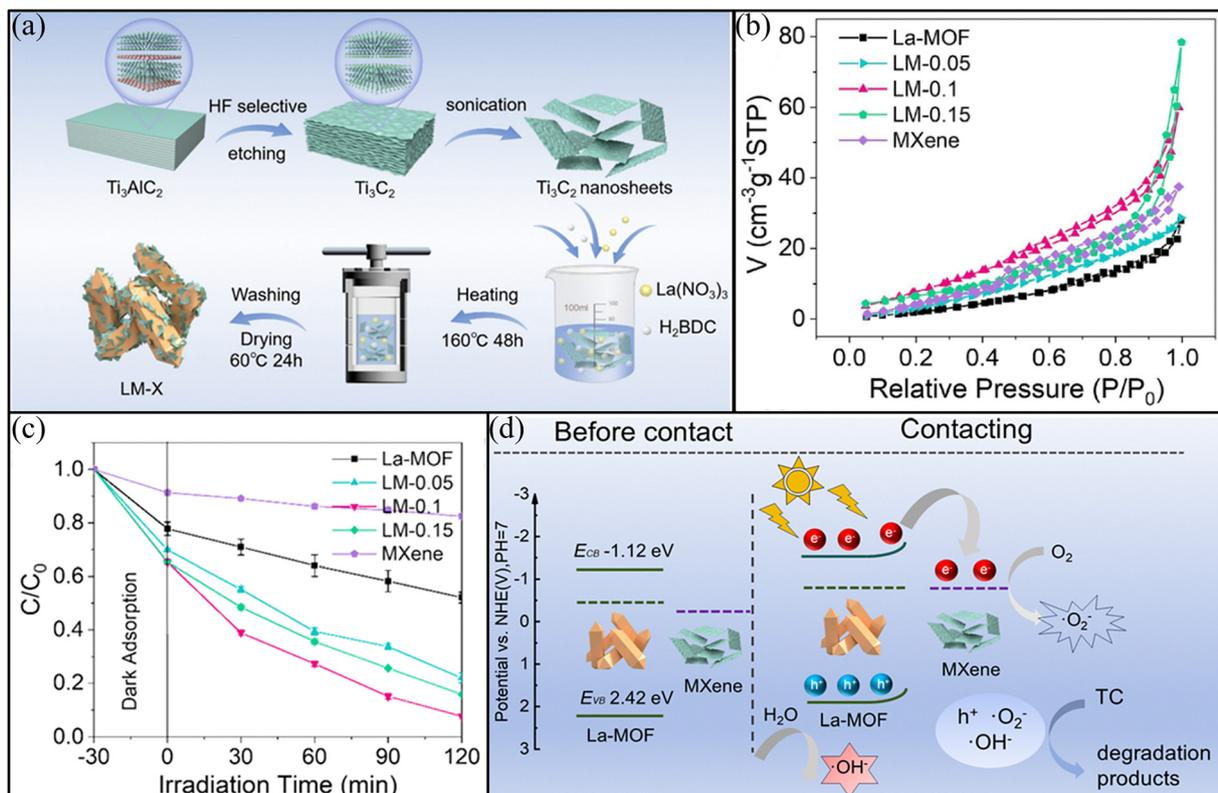
Fig. 7 (a) Schematic representation of the preparation of LM-0.1, (b)  $N_2$  adsorption–desorption isotherms, (c) TC removal with a xenon lamp and (d) possible method for degradation of TC by LM-0.1 under solar light exposure. Reproduced with permission from ref. 85. Copyright 2025, Elsevier.
