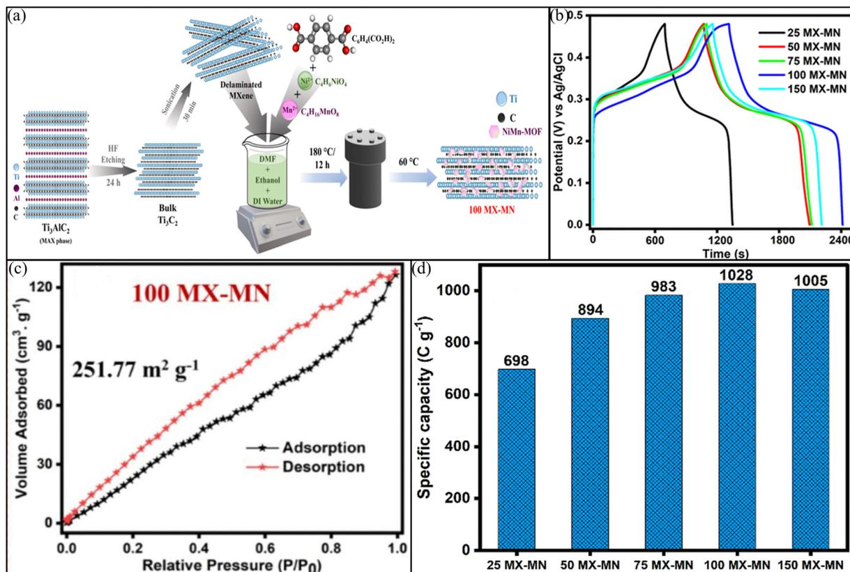
Fig. 19 (a) The schematic representation of etching aluminum from the MAX phase and the synthesis of composites. (b) The GCD curve at  $1 \text{ A g}^{-1}$ , (c) the nitrogen adsorption–desorption and pore distribution curves of the 100 MX-MN composite, and (d) specific capacity of all the composites at  $1 \text{ A g}^{-1}$ . Reproduced with permission from ref. 56. Copyright 2024, Elsevier.
