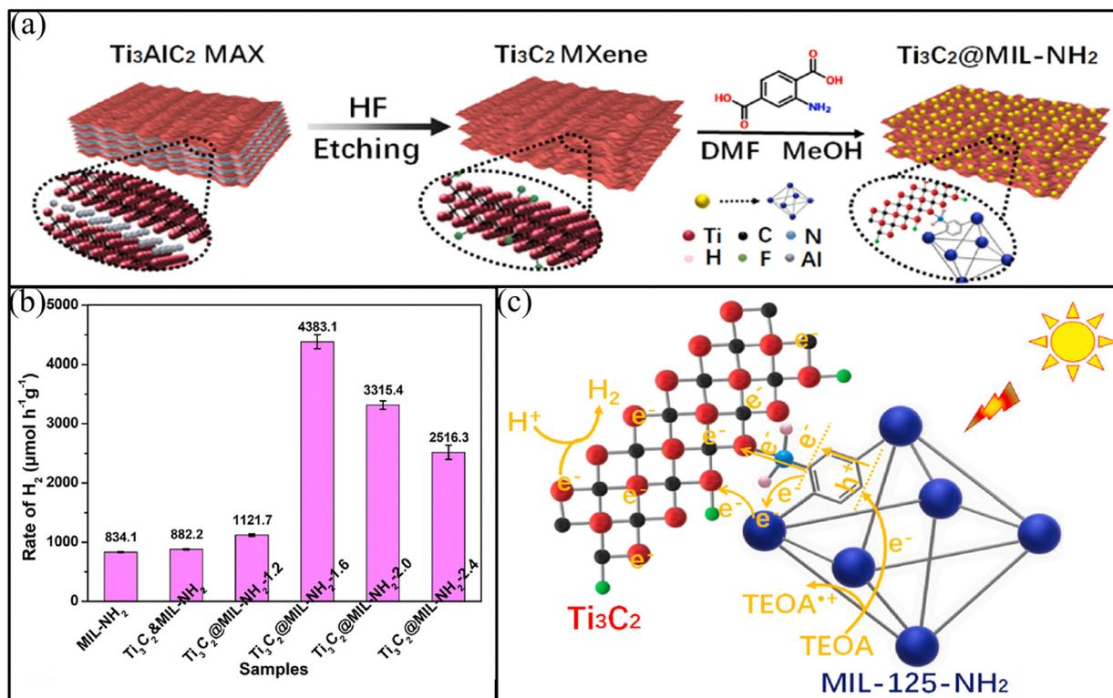
Fig. 12 (a) Schematic preparation process of Ti<sub>3</sub>C<sub>2</sub>@MIL-NH<sub>2</sub>, (b) H<sub>2</sub> production over the MIL-NH<sub>2</sub>, Ti<sub>3</sub>C<sub>2</sub>@MIL-NH<sub>2</sub> and Ti<sub>3</sub>C<sub>2</sub>@MIL-NH<sub>2</sub> composites, and (c) mechanism for H<sub>2</sub> production over the Ti<sub>3</sub>C<sub>2</sub>@MIL-NH<sub>2</sub> composite. Reproduced with permission from ref. 104. Copyright 2021, Elsevier.
