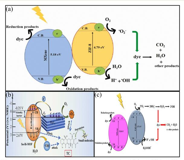
Fig. 11 (a) The degradation method by the MXOF nanocomposite. Reproduced with permission from ref. 69. Copyright 2023, Elsevier. (b) The suggested photocatalytic mechanism in Sn-Bi-MOF/Ti<sub>3</sub>C<sub>2</sub>.<sup>87</sup> (c) Schematic representation of MB and DR31 degradation mechanism using MXene@UiO-66 nanocomposite. Reproduced with permission from ref. 68. Copyright 2024, Elsevier.
