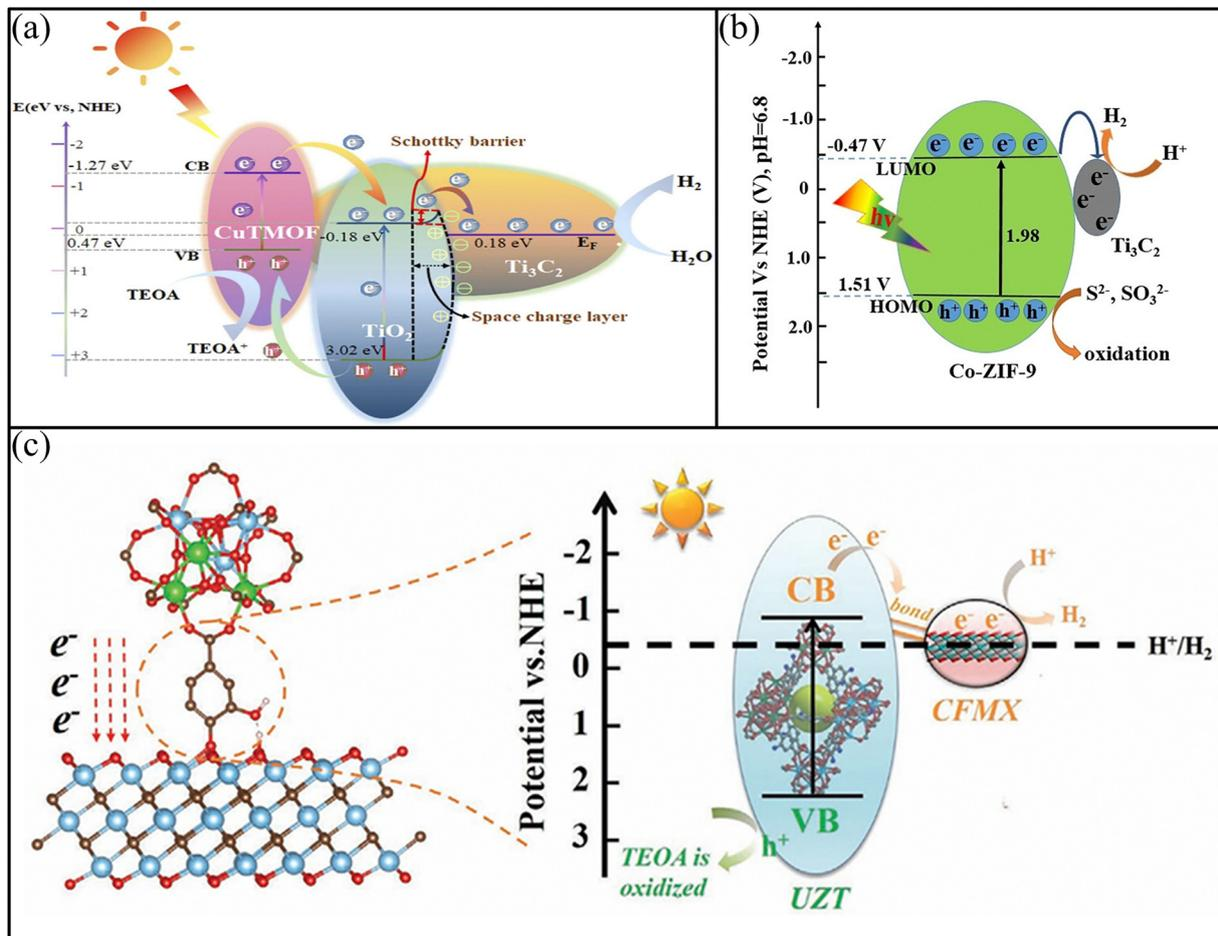
Fig. 16 (a) TT/CuTMOF nanocomposite photocatalytic mechanism. Reproduced with permission from ref. 107. Copyright 2023, Elsevier. (b) Possible photocatalytic mechanism for H<sub>2</sub>-evolution over the Co ZIF-9/Ti<sub>3</sub>C<sub>2</sub> composite. Reproduced with permission from ref. 105. Copyright 2022. (c) Schematic of the photocatalytic water splitting mechanism for UZT/CFMX. Reproduced with permission from ref. 101. Copyright 2022 open access CC BY 4.0.
