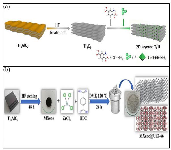
Fig. 4 (a) Schematic diagram for  $Ti_3C_2$  MXene and  $Ti_3C_2$ /UiO66NH<sub>2</sub> composite preparation. Figure reproduced from ref. 67, which is open access and permits unrestricted use of materials under the terms of the Creative Commons CC-BY. (b) Schematic depiction of the method for synthesizing of the MXene@UiO-66 nanocomposite. Reproduced with permission from ref. 68. Copyright 2024, Elsevier.
