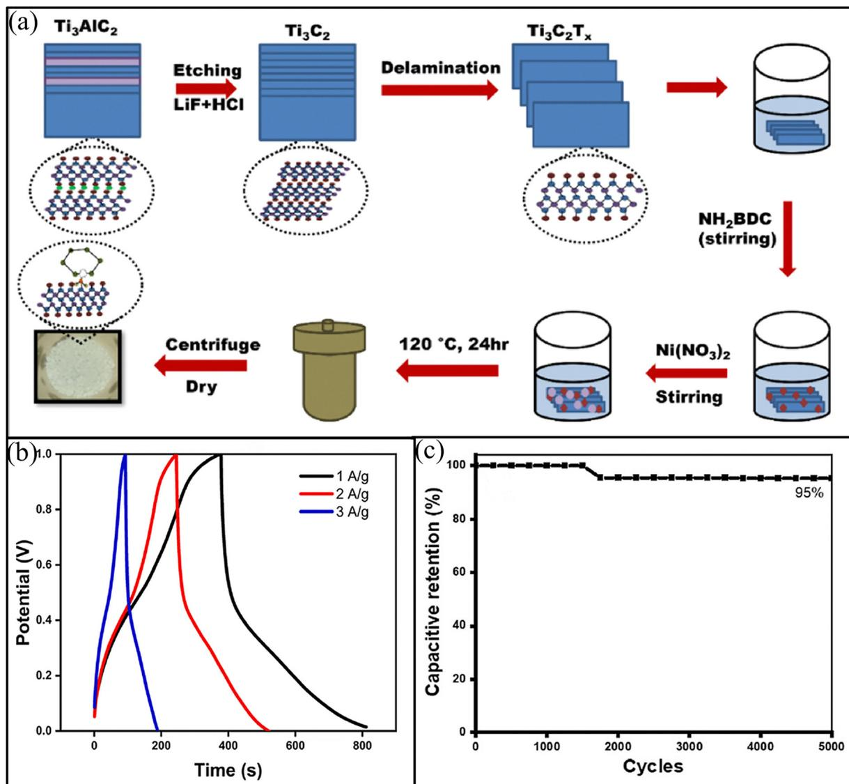
Fig. 18 (a) Schematic representation of the synthesis of the  $\text{Ti}_3\text{C}_2\text{T}_x/\text{Ni-MOF}$  composite, (b) GCD curve of the  $\text{Ti}_3\text{C}_2\text{T}_x/\text{Ni-MOF}$  composite at varied current densities, and (c) cycling stability performance of the device. Reproduced with permission from ref. 26. Copyright 2024, Elsevier.
