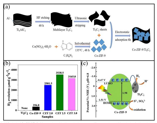
Fig. 14 (a) Synthesis of Co-ZIF-9/Ti $_3$ C $_2$ , (b) comparison of the H $_2$ -production rate over different samples, and (c) mechanism for H $_2$ -evolution over the Co-ZIF-9/Ti $_3$ C $_2$ . Reproduced with permission from ref. 105. Copyright 2022.
