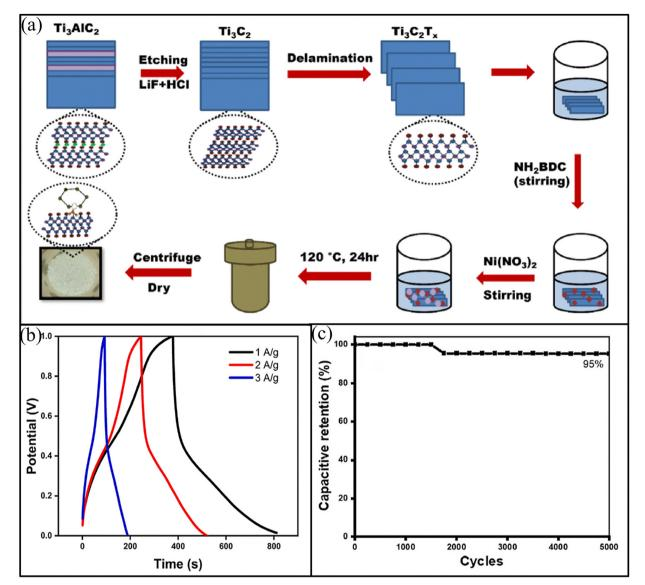
Fig. 18 (a) Schematic representation of the synthesis of the  $Ti_3C_2T_x/Ni$ -MOF composite, (b) GCD curve of the  $Ti_3C_2T_x/Ni$ -MOF composite at varied current densities, and (c) cycling stability performance of the device. Reproduced with permission from ref. 26. Copyright 2024, Elsevier.
