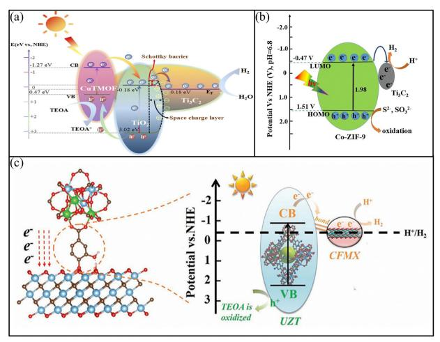
Fig. 16 (a) TT/CuTMOF nanocomposite photocatalytic mechanism. Reproduced with permission from ref. 107. Copyright 2023, Elsevier. (b) Possible photocatalytic mechanism for  $H_2$ -evolution over the Co ZIF-9/ $Ti_3C_2$  composite. Reproduced with permission from ref. 105. Copyright 2022. (c) Schematic of the photocatalytic water splitting mechanism for UZT/CFMX. Reproduced with permission from ref. 101. Copyright 2022 open access CC
