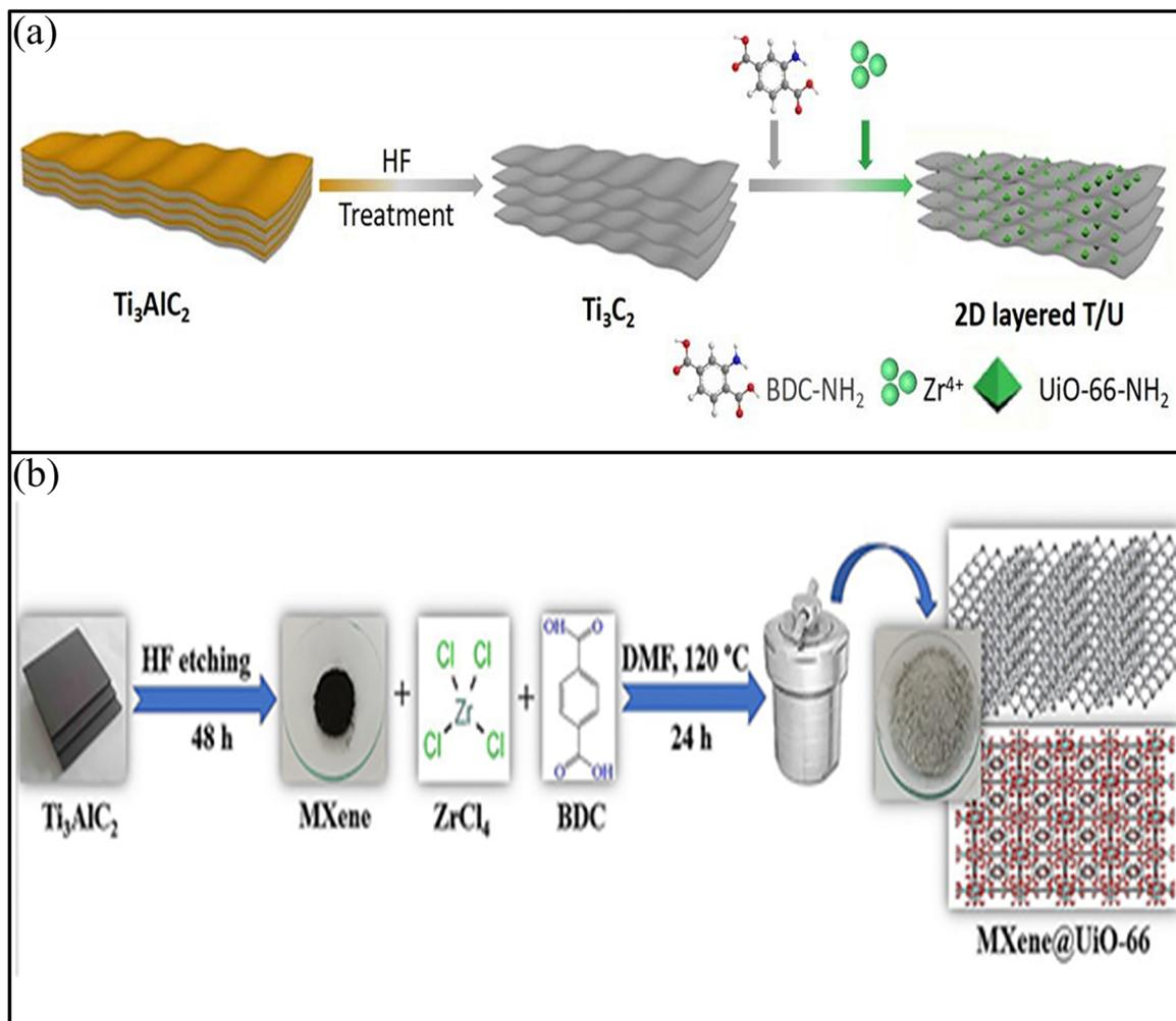
Fig. 4 (a) Schematic diagram for  $\text{Ti}_3\text{C}_2$  MXene and  $\text{Ti}_3\text{C}_2/\text{UiO}66\text{NH}_2$  composite preparation. Figure reproduced from ref. 67, which is open access and permits unrestricted use of materials under the terms of the Creative Commons CC-BY. (b) Schematic depiction of the method for synthesizing of the MXene@UiO-66 nanocomposite. Reproduced with permission from ref. 68. Copyright 2024, Elsevier.
