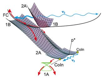
Fig. 2 Potentials, wave packet paths and coherent oscillations according to ref. 12. FC is the Franck-Condon region, p\* the pericyclic minimum. The molecular structures at the two Colns are indicated in Fig. 1. The oscillation leading to periodic bond splitting is  $\nu_3$  (140 cm<sup>-1</sup>, period 240 fs), the lifetime (traveling time) in 2A is 80 fs.
