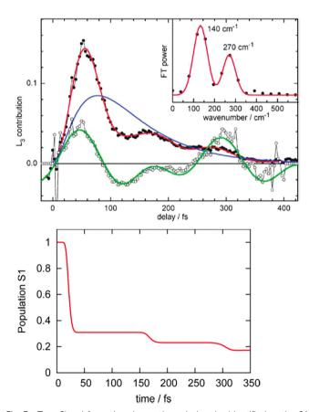
Fig. 3 Top: Signal from the observation window L<sub>3</sub>, identified as the 2A  $(S_1)$  surface (black dots), which can be simulated by the product of an exponential part (dark blue solid line) with an oscillatory part (Fourier transform in the inset); the 270 cm<sup>-1</sup> band was ascribed to an overtone of that at 140 cm<sup>-1</sup> (from ref. 12). Bottom: Calculated 2A populations, showing the steps, when the wave packet comes close to a Coln (from ref. 13, with permission of ACS).
