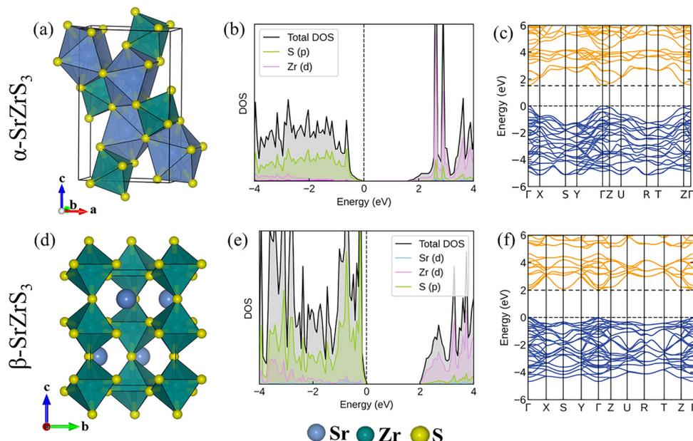
Fig. 1 (a) and (d) Optimized crystal structures, (b) and (e) projected density of states (PDOS), and (c) and (f) band structures of  $\alpha$ -SrZrS<sub>3</sub> and  $\beta$ -SrZrS<sub>3</sub> perovskites.
