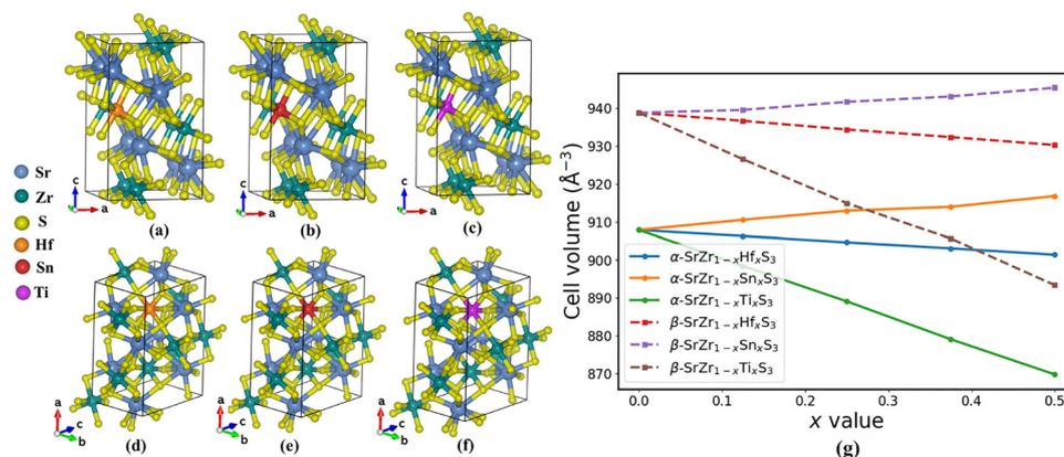
Fig. 2 Optimized structures of (a) and (d)  $\alpha$ - and  $\beta$ -SrZr<sub>1-x</sub>Hf<sub>x</sub>S<sub>3</sub>, (b) and (e)  $\alpha$ - and  $\beta$ -SrZr<sub>1-x</sub>Sn<sub>x</sub>S<sub>3</sub>, and (c) and (f)  $\alpha$ - and  $\beta$ -SrZr<sub>1-x</sub>Ti<sub>x</sub>S<sub>3</sub>. (g) Variation of supercell volume with doping concentration  $x$ . Supercell sizes for the  $\alpha$ - and  $\beta$ -phases are  $1 \times 2 \times 1$  and  $2 \times 1 \times 1$ , respectively.
