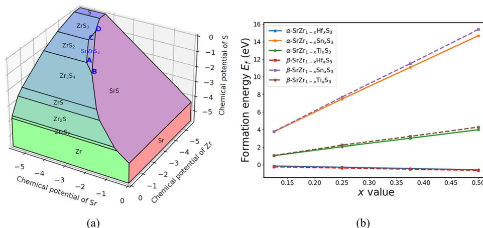
Fig. 8 (a) Thermodynamically stable region of SrZrS<sub>3</sub> in the Sr–Zr–S system. (b) Substitutional defect formation energies of α- and β-SrZr<sub>1-x</sub>Hf<sub>x</sub>S<sub>3</sub>, SrZr<sub>1-x</sub>Sn<sub>x</sub>S<sub>3</sub>, and SrZr<sub>1-x</sub>Ti<sub>x</sub>S<sub>3</sub>.
