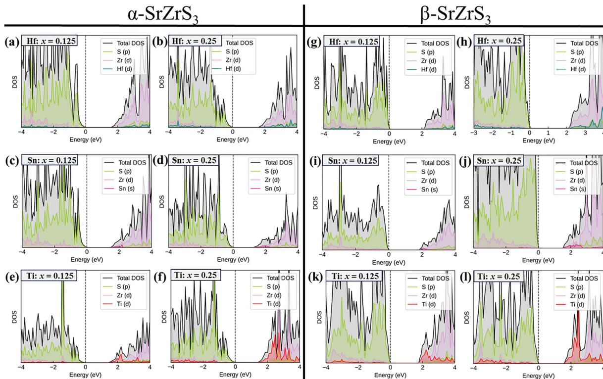
Fig. 4 Projected density of states (PDOS) of (a–f)  $\alpha$ - and (g–l)  $\beta$ -phase  $\text{SrZr}_{1-x}\text{Hf}_x\text{S}_3$ ,  $\text{SrZr}_{1-x}\text{Sn}_x\text{S}_3$ , and  $\text{SrZr}_{1-x}\text{Ti}_x\text{S}_3$  ( $x = 0.125$  and  $0.25$ ).
