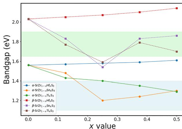
Fig. 5 Variation of the band gaps of  $\alpha$ - and  $\beta$ - $\text{SrZr}_{1-x}\text{Hf}_x\text{S}_3$ ,  $\text{SrZr}_{1-x}\text{Sn}_x\text{S}_3$ , and  $\text{SrZr}_{1-x}\text{Ti}_x\text{S}_3$  with the doping concentration  $x$ .
