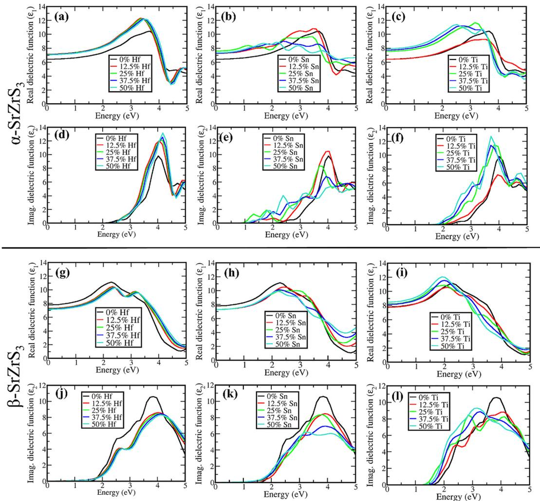
Fig. 6 Real and imaginary parts of the dielectric functions of (a–f)  $\alpha$ - and (g–l)  $\beta$ -phase  $\text{SrZr}_{1-x}\text{Hf}_x\text{S}_3$ ,  $\text{SrZr}_{1-x}\text{Sn}_x\text{S}_3$ , and  $\text{SrZr}_{1-x}\text{Ti}_x\text{S}_3$ .
