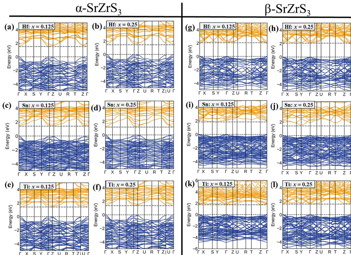
Fig. 3 Electronic band structures of (a–f)  $\alpha$ - and (g–l)  $\beta$ -phase  $\text{SrZr}_{1-x}\text{Hf}_x\text{S}_3$ ,  $\text{SrZr}_{1-x}\text{Sn}_x\text{S}_3$ , and  $\text{SrZr}_{1-x}\text{Ti}_x\text{S}_3$  ( $x = 0.125$  and  $0.25$ ) materials.
