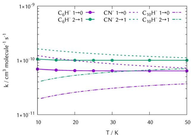
Fig. 12 Comparison between calculated inelastic rate coefficients for collisions of the  $C_{10}H^-$  anion with He, and those obtained earlier in ref. 37 for the  $C_6H^-$  anion. Results for other species reported in ref. 37 are also shown. See the main text for discussion.
