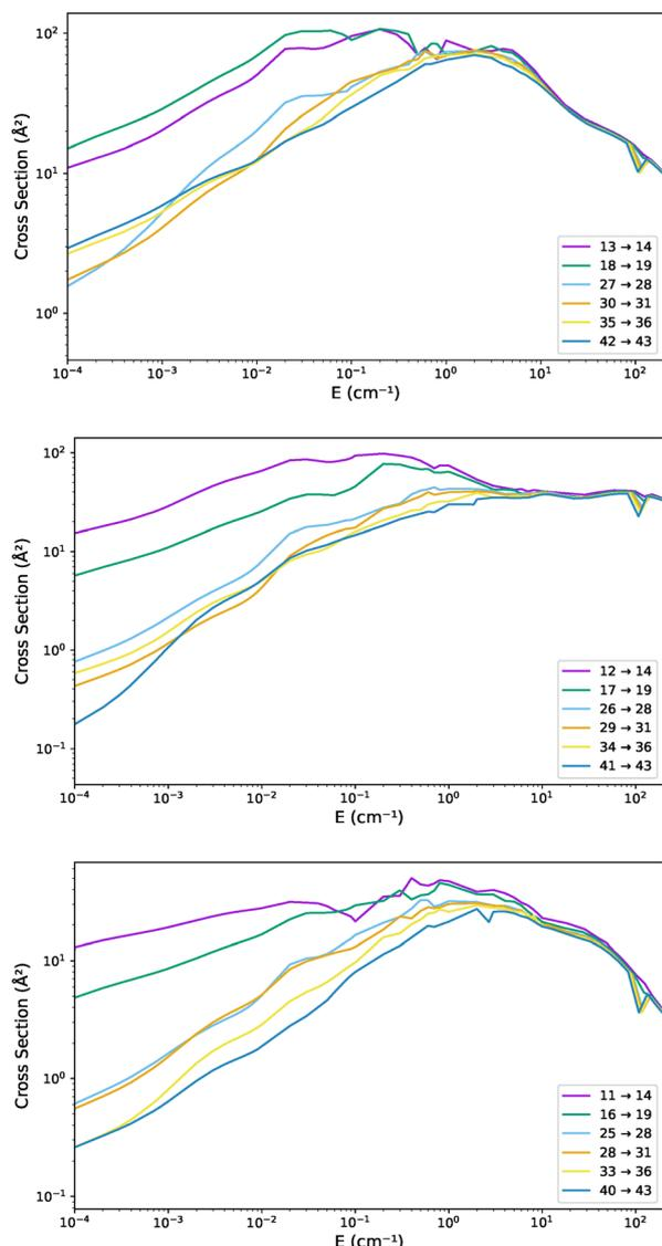
Fig. 9 The panels of this figure report excitation rotational cross sections for the title anion of this work in collision with He atoms. The top panel shows  $\Delta j = +1$  transitions, while the middle panel shows the  $\Delta j = +2$  processes and the bottom panel the  $\Delta j = +3$  excitations. See the main text for further comments.
