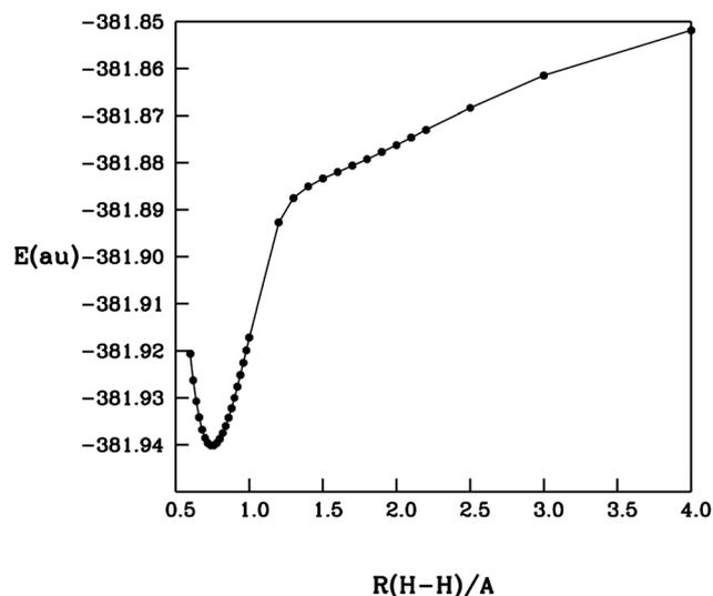
Fig. 3 Detailed energy region around the products' formation. The minimum energy corresponds to the equilibrium geometry of the newly formed  $\text{H}_2$  molecule with the molecular anion located further away. Distances in Å and energies in a.u. The  $R(\text{H}-\text{H})$  distance is the same as in Fig. 2. See main text for further details.
