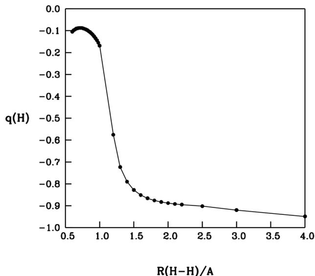
Fig. 4 Evolution of the extra negative charge on the incoming  $\text{H}^-$  atom as it approaches the neutral radical and the  $\text{H}_2$  neutral molecule is formed while the negative charge moves onto the product anion (not shown). The  $R(\text{H}-\text{H})$  variable shows the distance between the H anion and the terminal H atom of the neutral. All distances in Å. See main text for further details.
