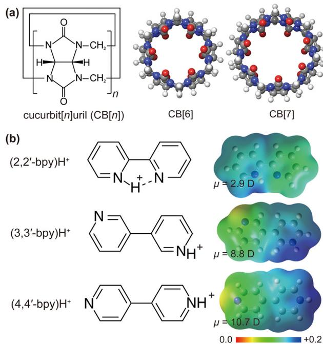
**Fig. 1** (a) Structures of cucurbit[*n*]urils (*n* = 6 and 7), and (b) protonated *n,n'*-bipyridines (**nbpy**·H<sup>+</sup>, *n* = 2, 3, and 4) and their electrostatic potential map. The region mapped with blue surface represents the positively charged area. The dipole moments ( $\mu$ , unit: Debye) of protonated bipyridines are given as well.
