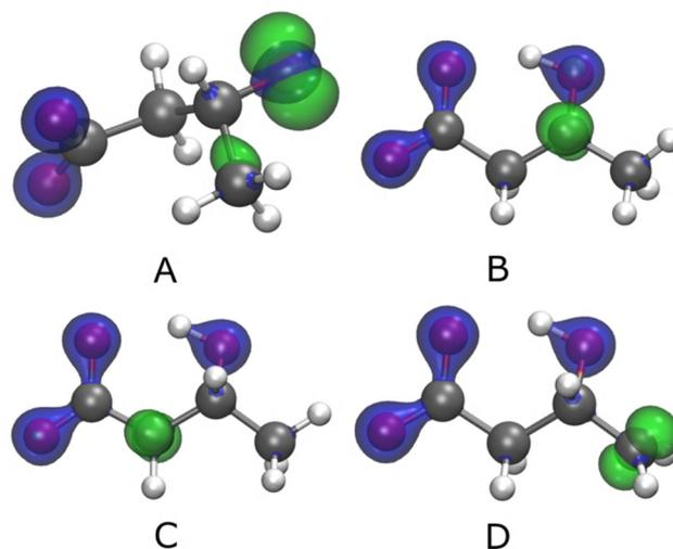
**Fig. 5** (A) Distribution of charge (blue) and spin (green) in radicals formed by hydrogen abstraction. (A) PCET at O1–H8. (B) HAT at C2–H9. (C) HAT at C3–H10 (also representative of HAT at C3–H11). (D) HAT at C7–H12 (also representative of HAT at C7–H13 and C7–H14). The density isosurface was rendered at 0.3 a.u. (for charge) and 0.03 a.u. (for spin).
