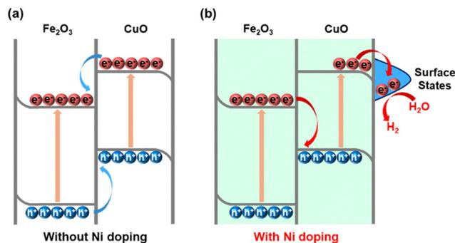
Fig. 6 Diagram of the photocatalytic water cracking mechanism of photocatalysts for CFO500 (a) and CFO500-2%Ni (b).
