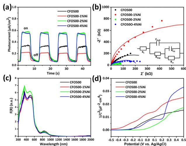
Fig. 3 (a) *I*-*t* curves; (b) EIS Nyquist plots under illumination; (c) transformed Kubelka–Munk reflectance spectra of CFO materials; (d) Mott–Schottky plots of CFO500, CFO500-1%Ni, CFO500-2%Ni and CFO500-4%Ni.
