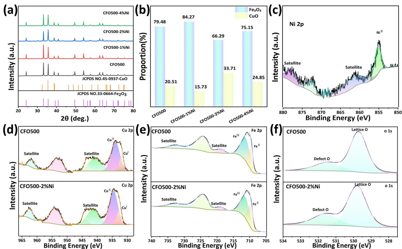
Fig. 2 (a) XRD patterns of CFO500, CFO500-1%Ni, CFO500-2%Ni and CFO500-4%Ni; (b) refined phase composition of CFO; (c) Ni 2p spectrum of CFO500-2%Ni; (d) Cu 2p spectra of CFO500 and CFO500-2%Ni; (e) Fe 2p spectra of CFO500 and CFO500-2%Ni; (f) O 1s spectra of CFO500 and CFO500-2%Ni.
