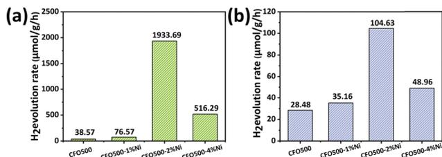
Fig. 5 (a) The catalytic activity of gas products of different samples under the illumination of a 10 W ultraviolet light with a wavelength of 355 nm; (b) the catalytic activity of gas products of different samples under the illumination of a 10 W LED light.
