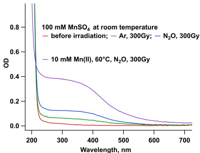
Fig. 5 Absorption spectra of products observed after pulse radiolysis in Ar- and N<sub>2</sub>O-saturated solutions with 100 mM MnSO<sub>4</sub> at pH 5 at room temperature, as well as in 10 mM MnSO<sub>4</sub> solutions at 60 °C.
