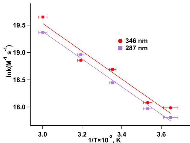
Fig. 3 The natural logarithm of the second-order rate constants measured at 346 nm and 287 nm for the reaction of Mn(II) with H atoms is plotted against the inverse temperature for MnSO<sub>4</sub> solutions at pH 3, over a temperature range from 1 °C to 60 °C. Arrhenius plot fit results are shown by the solid line ( $\ln k_{0(346\text{nm})} = -2549/T + 27.2$ ;  $\ln k_{0(287\text{nm})} = -2532/T + 27.0$ ).
