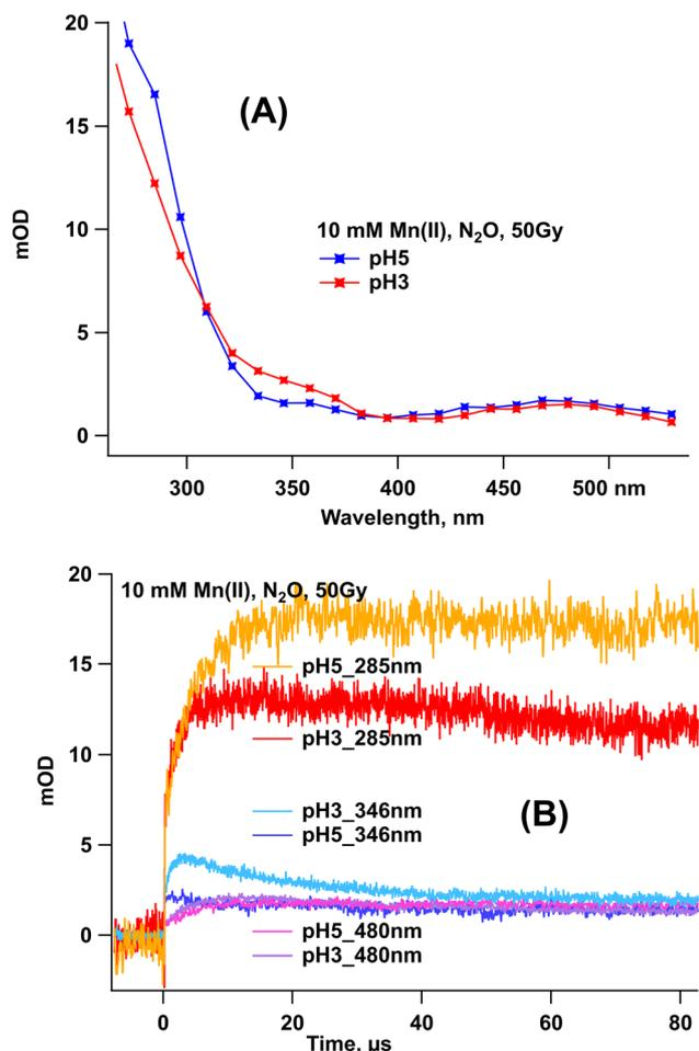
Fig. 4 Transient absorption spectra (A) and the kinetics at various wavelengths (B) observed 50  $\mu$ s after 15-ns pulse radiolysis (50 Gy) in  $N_2O$ -saturated  $MnSO_4$  solutions at pH 5 and 3 at room temperature.
