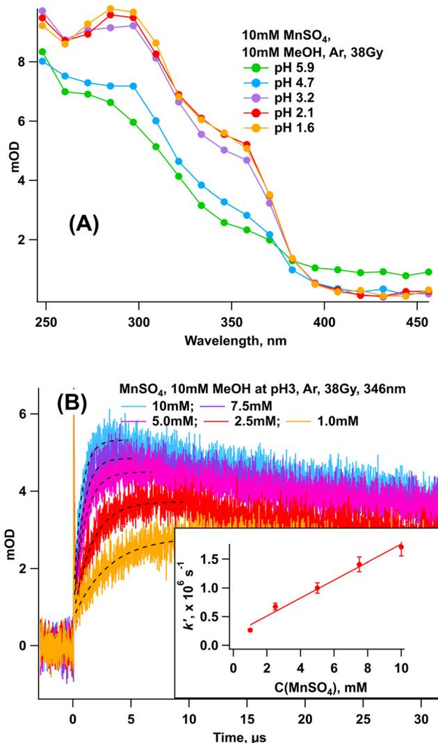
Fig. 2 Transient absorption spectra (A) and kinetics at 346 nm (B) observed 5  $\mu$ s after 12-ns pulse radiolysis (38 Gy) in Ar-saturated  $\text{MnSO}_4$  solutions at different pH at room temperature. ((B), insert) Pseudo-first-order rate constants ( $k'$ ) plotted against the  $\text{MnSO}_4$  concentration to obtain second-order rate constants.
