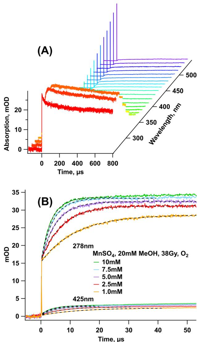
Fig. 6 Transient absorption spectra (A) and the kinetics at 278 and 425 nm (B) observed after 15-ns pulse radiolysis (38 Gy) in O<sub>2</sub>-saturated MnSO<sub>4</sub> solutions with 20 mM MeOH at pH 5 at room temperature.
