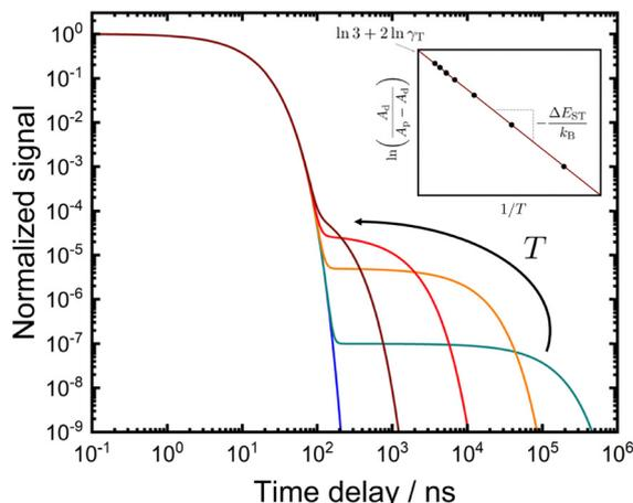
**Fig. 3** Schematic temperature-dependent decay curves of the excited singlet state  $S_1$  of a typical TADF emitter within the weak coupling scheme ( $k_p = 0.1 \text{ ns}^{-1}$ ,  $k_d$  in  $\mu\text{s}^{-1}$  range). The inset depicts the behavior of the amplitude of the delayed component according to eqn (15) that could be used to calibrate the emitter for ratiometric thermometry in the time domain.
