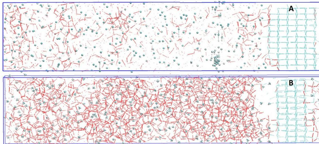
Fig. 4 The case of collective stochastic nucleation using 15.0 mol% methane concentration: (A) multiple nuclei formations are observed at the same time ( $t = 1$  ns) and later (B) convert into the crystalline structure (end of 500 ns). Three layers of ice have been melted, indicating a shrinking core mechanism when methane is excessive.<sup>64</sup>
