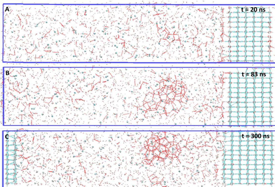
Fig. 3 The promoted nucleation of methane hydrate from an initial 5.8 mol% CH<sub>4</sub> aqueous solution. The snapshot taken before the nucleation (A), with nucleus reaching the critical size MCG1 = 16 (B) and coupled growth of ice and hydrate at the end of 300 ns (C).
