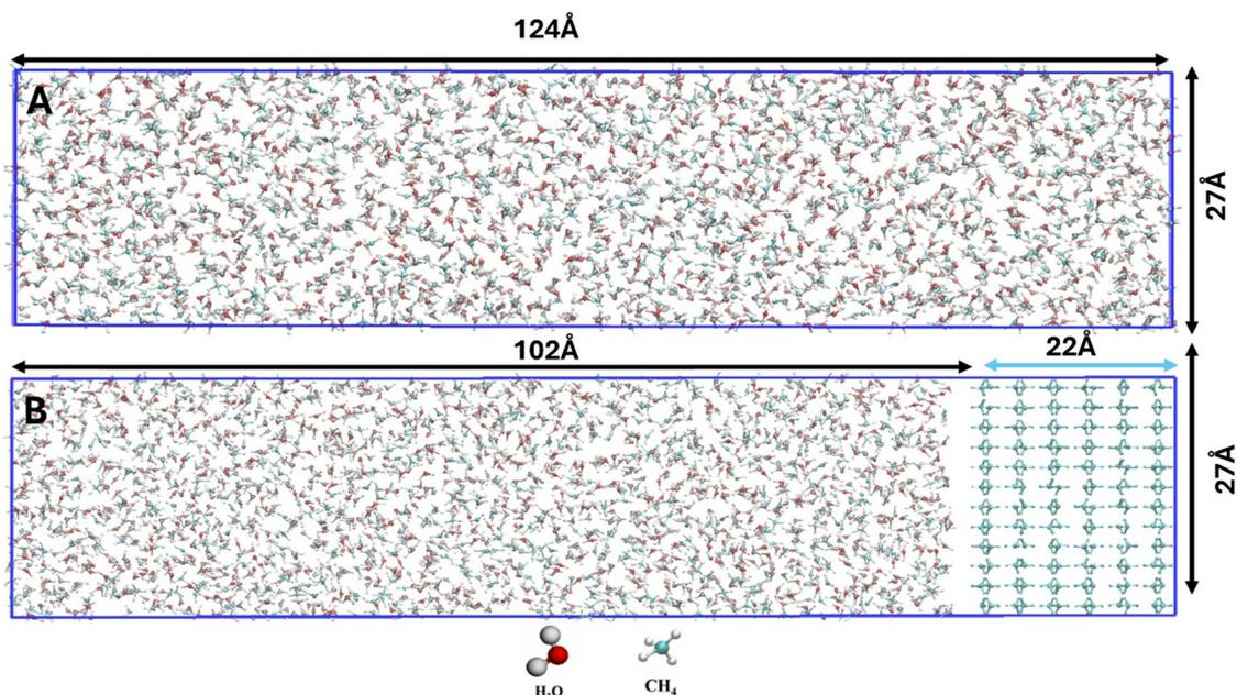
Fig. 1 The initial simulation configurations of (A) the reference homogeneous aqueous methane solution and (B) the heterogeneous system of the solution in contact with the basal surface of hexagonal ice Ih ( $6 \times 3 \times 3$  lattice, 432 H<sub>2</sub>O molecules). Water and methane molecules are presented in their respective colors. All systems are run at 250 K and 50 MPa and a variable initial aqueous methane mole fraction from 3.0 to 15.0%.
