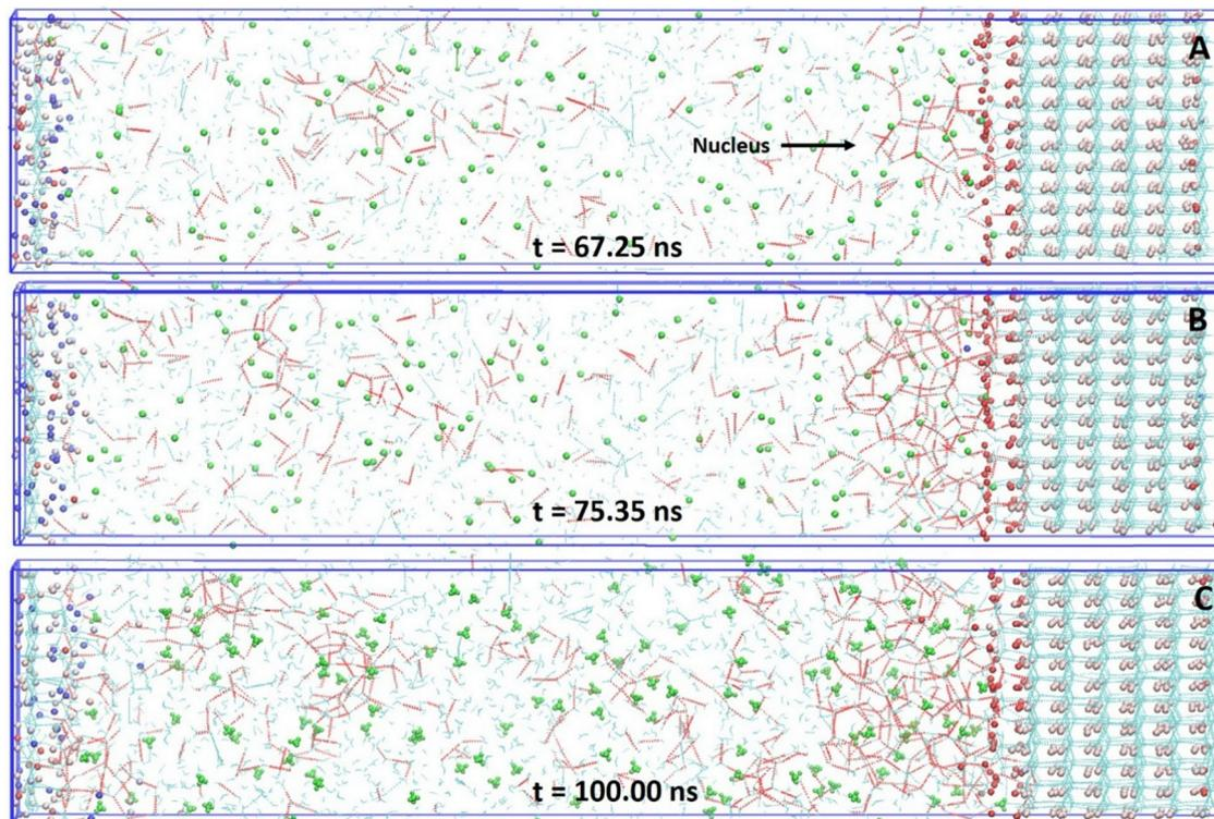
Fig. 6 (A) Surface nucleation case (6.25 mol%  $\text{CH}_4$ ) at 67.25 ns, where cubic ice (red color) is formed to initiate nucleation and (B) and (C) further growth at 75.35 ns onwards and hydrates stick to the ice surface. Hexagonal ice, cubic ice and methane hydrate are shown in this figure by silver, red and blue colors, respectively. Methane gas molecules are shown in green color.
