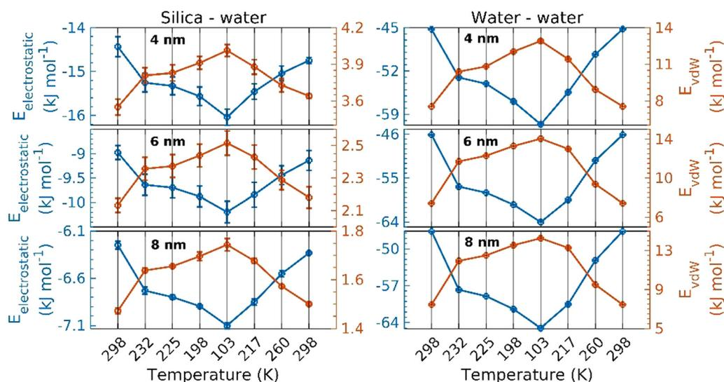
**Fig. 9** Variation of the non-bonding interaction energies (electrostatic ( $E_{\text{electrostatic}}$ ) and van der Waals ( $E_{\text{vdW}}$ )) in silica–water and water–water combinations normalized by the number of water molecules in each system as a function of the control temperatures used in the simulations of neat water systems of pore width 4, 6, and 8 nm. The standard deviations are obtained from triplicates of each simulation.
