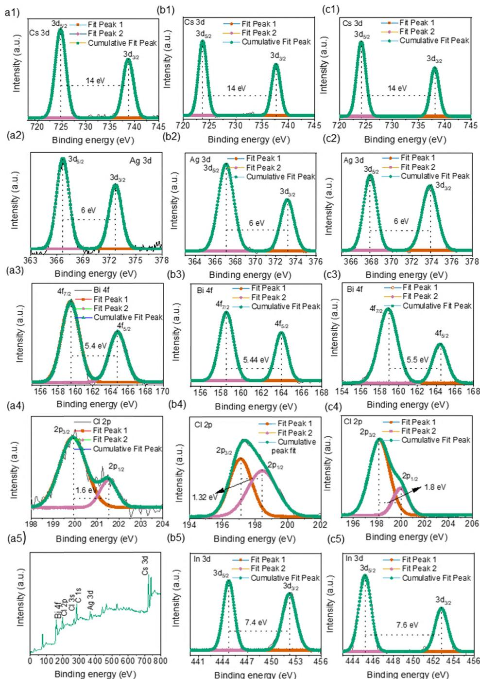
Fig. 2 (a1)–(a5) Narrow scan and survey scan XPS spectra of the  $\text{Cs}_2\text{AgIn}_x\text{Bi}_{1-x}\text{Cl}_6$  ( $x = 0$ ) sample. (b1)–(b5) Narrow scan XPS spectra of the  $\text{Cs}_2\text{AgIn}_x\text{Bi}_{1-x}\text{Cl}_6$  ( $x = 0.5$ ) sample. (c1)–(c5) Narrow scan XPS spectra of the  $\text{Cs}_2\text{AgIn}_x\text{Bi}_{1-x}\text{Cl}_6$  ( $x = 0.75$ ) sample.
