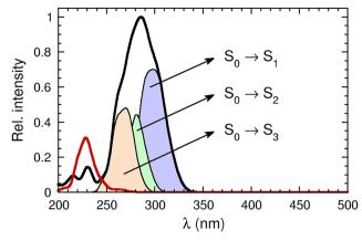
Fig. 2 XMS-CASPT2/cc-pVTZ UV-vis absorption spectrum of amineboranes 1a (red curve) and 1b (black curve), and the individual contributions of the three lowest-lying singlet states of 1b. No absorption is observed above 500 nm in any case.
