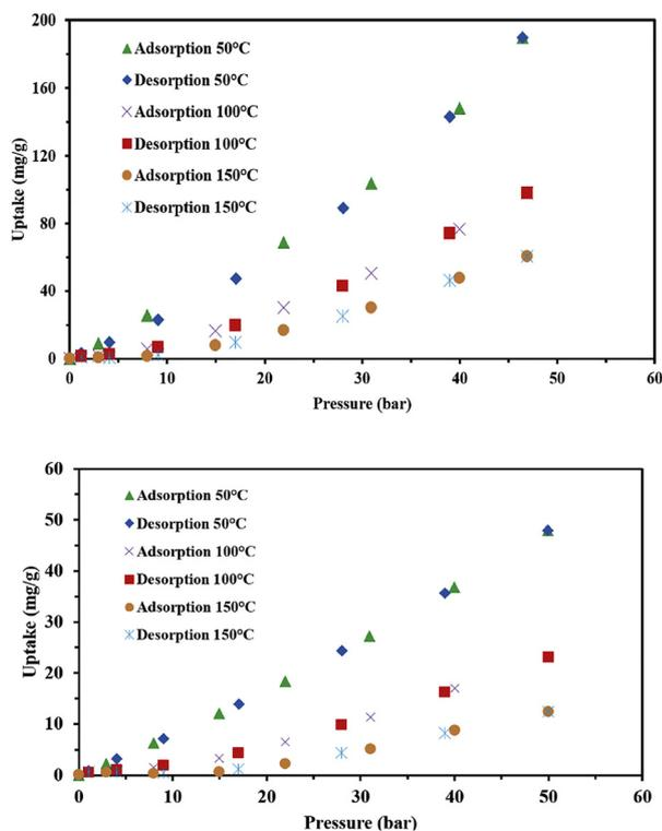
Fig. 18 Evolution with temperature and pressure of the adsorption and desorption of CO<sub>2</sub> (top) and CH<sub>4</sub> (below) on carbonate rocks. Adapted from ref. 52 with permission from Elsevier B. V., copyright 2018.
