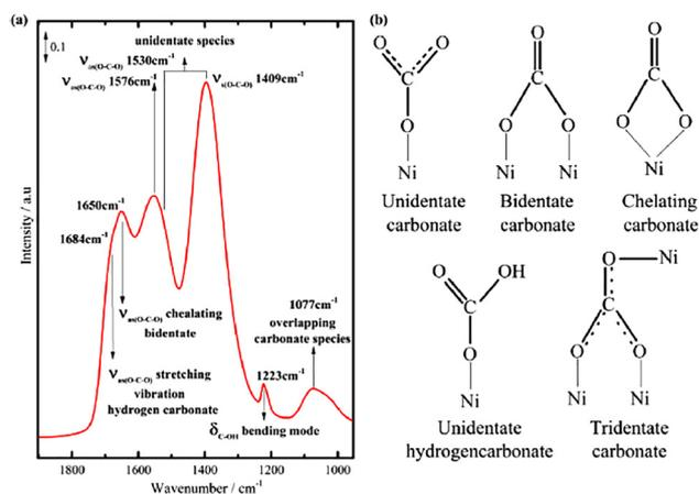
Fig. 13 (a) Infrared spectra of CO<sub>2</sub> adsorbed on the Ni-hydrotalcite derived catalyst and (b) possible species appeared in the CO<sub>2</sub> adsorption experiment. Adapted from ref. 38 with permission from Elsevier B. V., copyright 2023.
