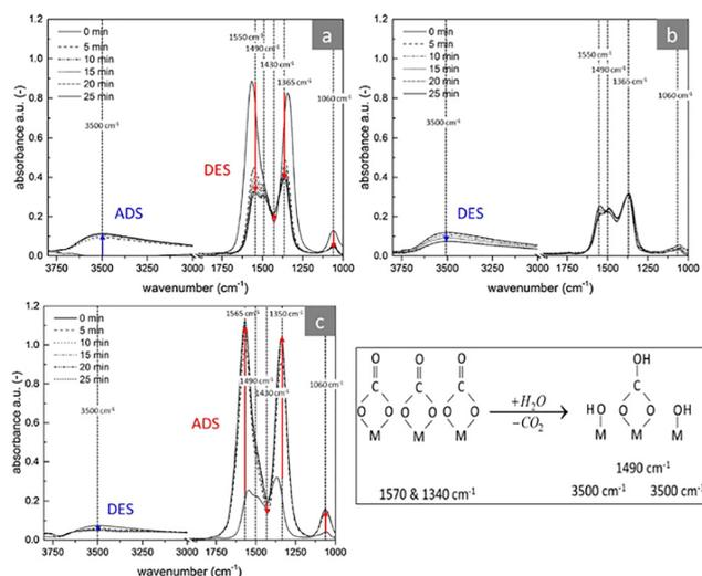
Fig. 15 IR spectra of hydrotalcite after (a) adsorption of  $\text{H}_2\text{O}$  at 400 °C, (b) desorption of  $\text{H}_2\text{O}$  at 400 °C with  $\text{N}_2$  and (c) adsorption of  $\text{CO}_2$  at 400 °C after desorption with  $\text{H}_2\text{O}$  and  $\text{N}_2$ . The equation shows  $\text{H}_2\text{O}$  adsorption and  $\text{CO}_2$  liberation. Adapted from ref. 1 with permission from Elsevier B. V., copyright 2018.
