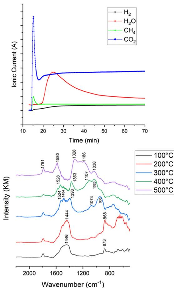
Fig. 12 Operando CO<sub>2</sub> methanation at 400 °C on Ni/dolomite: (Top) evolution of mass spectroscopy signal with reaction time. (Bottom) *In situ* DRIFT spectra as a function of catalyst temperature. Adapted from ref. 37 with permission from Elsevier B. V., copyright 2024.
