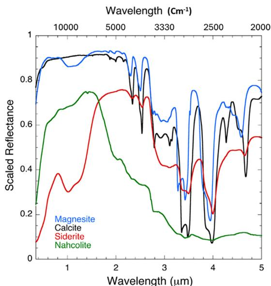
Fig. 4 NIR reflectance spectra (at  $2000\text{--}28\,571\text{ cm}^{-1}$ ) of anhydrous carbonates: calcite, magnesite, siderite, and nahcolite. Adapted from ref. 21 with permission from Elsevier B. V., copyright 2015.
