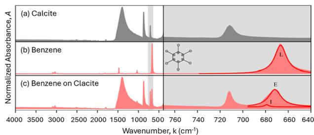
Fig. 16 [Left] IR spectra at 400–4000  $\text{cm}^{-1}$  of (a) calcite, (b) benzene, and (c) benzene on calcite. [Right] Expanded view of 640–770  $\text{cm}^{-1}$ . L: liquid, E: extended adsorption layers, I: first adsorption layer. Adapted from ref. 50 with permission from American Chemical Society, copyright 2015.
