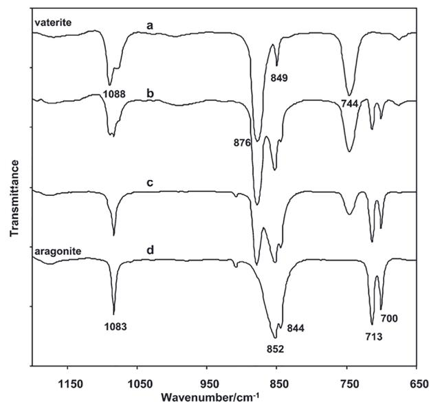
Fig. 8 FTIR spectra ( $650\text{--}1200\text{ cm}^{-1}$ ) of (a) the vaterite sample, and when it was refluxed in distilled water for (b) 30 min, (c) 60 min, and (d) 75 min. Adapted from ref. 27 with permission from American Chemical Society, copyright 2010.
