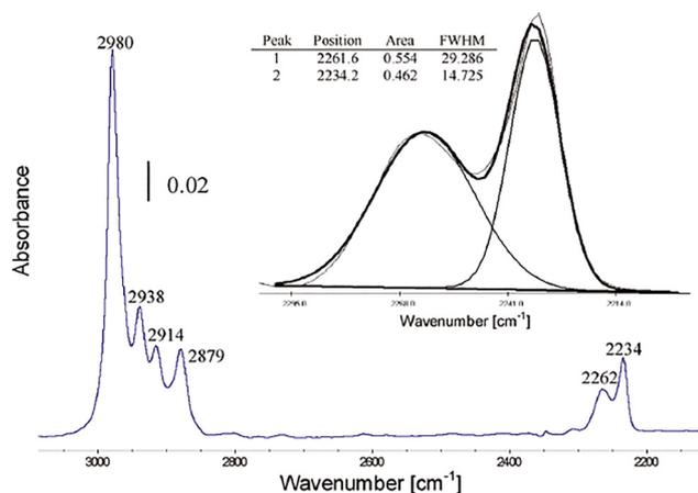
Fig. 17 *Tert*-Butyl cyanide adsorption on carbonated MgO activated at 240 °C. The zoom-in region of 2300–2150 cm<sup>-1</sup>. The deconvolution results are shown in the inset. Adapted from ref. 4 with permission from American Chemical Society, copyright 2011.
