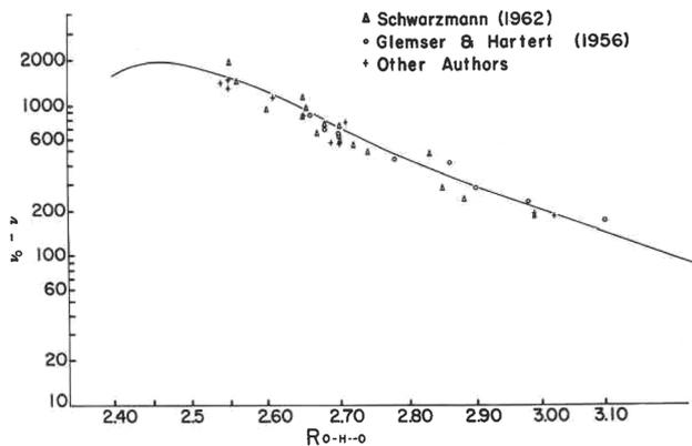
Fig. 9 Relationship between the O–H frequency ( $\nu$ ) and O–H...O distance in H-bonds ( $R_{\text{O-H}\cdots\text{O}}$ ); where  $\nu_0 = 3756 \text{ cm}^{-1}$  on the Y-axis. Adapted from ref. 28 with permission from Mineralogical Society of America, copyright 1971.
