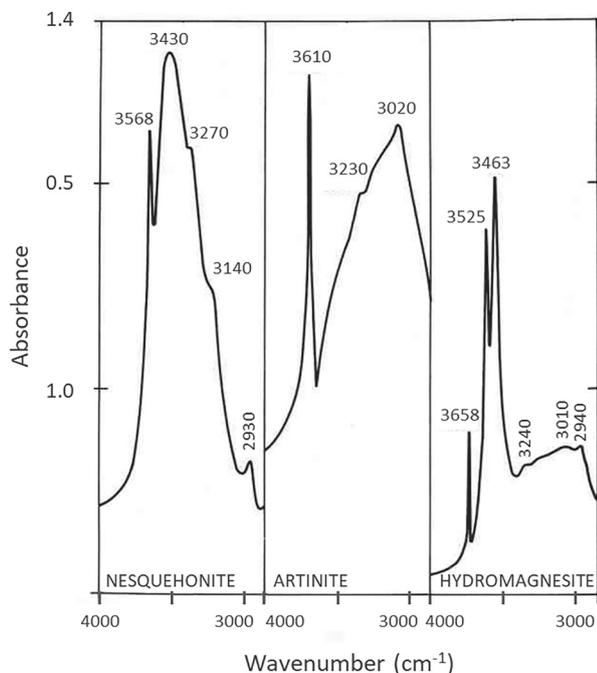
Fig. 10 Spectra of the hydrous magnesium carbonate minerals in the near infrared. Adapted from ref. 28 with permission from Mineralogical Society of America, copyright 1971.
