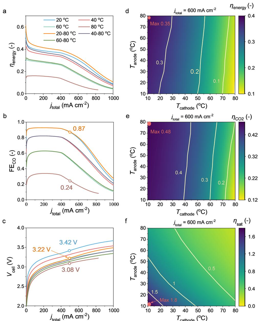
Fig. 3  $\eta_{\text{energy}}$  (a),  $\text{FE}_{\text{CO}_2}$  (b), and (c)  $V_{\text{cell}}$  as a function of  $j_{\text{total}}$  for different temperature cases. (d) Contour maps of  $\eta_{\text{energy}}$  (d),  $\eta_{\text{CO}_2}$  (e), and  $\eta_{\text{sat}}$  (f), as a function of various combinations of  $T_{\text{anode}}$  and  $T_{\text{cathode}}$  at  $600 \text{ mA cm}^{-2}$ .
