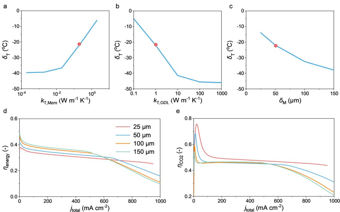
Fig. 5 (a) Impact of varying thermal conductivities ( $k_{\text{T,Mem}}$ ) of the AEM (a), thermal conductivities ( $k_{\text{T,GDL}}$ ) of the GDL (b) and AEM thicknesses ( $\delta_{\text{M}}$ ) (c) on the average temperature difference between the anode catalyst layer (aCL) and the cathode catalyst layer (cCL).  $\eta_{\text{energy}}$  (d) and  $\eta_{\text{CO}_2}$  (e) as a function of  $j_{\text{total}}$  for different AEM thickness cases.
