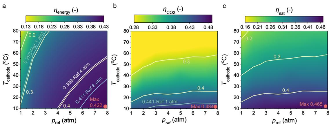
Fig. 6 Contour plots of  $\eta_{\text{energy}}$  (a),  $\eta_{\text{CO}_2}$  (b), and  $\eta_{\text{sat}}$  (c), as a function of various combinations of  $p_{\text{ref}}$  and  $T_{\text{cathode}}$  at  $T_{\text{anode}} = 80$  °C and  $j_{\text{total}} = 600$  mA cm $^{-2}$ .
