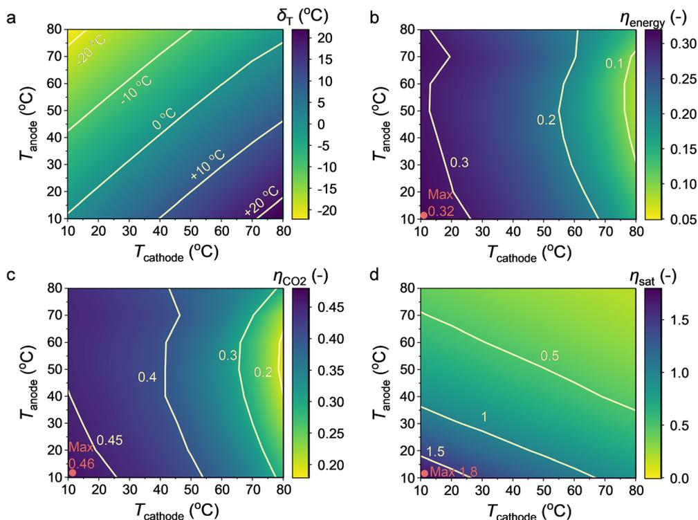
Fig. 4 Simulated temperature differences considering realistic heat transfer for various temperature combinations (a); contour plots of  $\eta_{\text{energy}}$  (b),  $\eta_{\text{CO}_2}$  (c), and  $\eta_{\text{sat}}$  (d) as a function of set  $T_{\text{anode}}$  and  $T_{\text{cathode}}$ , at  $600 \text{ mA cm}^{-2}$  under realistic heat transfer conditions.
