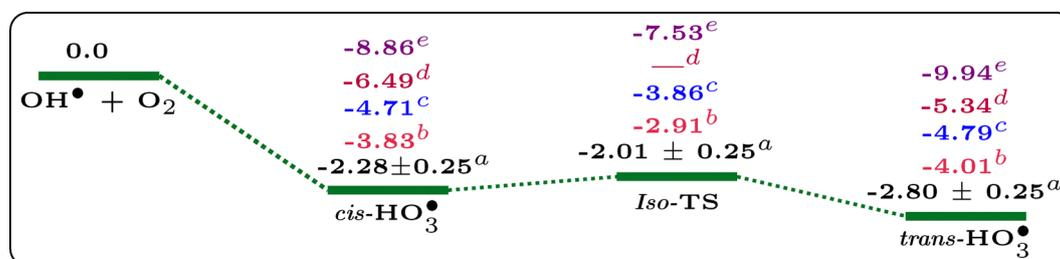
Fig. 1 Comparison of the four potential energy surfaces for  $\text{HO}_3^\bullet$  (ZPE-uncorrected) developed by: (e) Braams and Hua-Gen Yu,<sup>21</sup> (d) Hua-Gen Yu and Varandas,<sup>20</sup> (c) Xixi Hu *et al.*,<sup>22</sup> and (b) J. Zuo *et al.*,<sup>23</sup> with benchmark calculations from (a) Bartlett *et al.*<sup>10</sup> The benchmark results of Bartlett *et al.* are ZPE-corrected.
