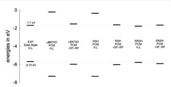
Fig. 2 Anthracene PCM-calculated HOMO, LUMO (H,L) energies, and -OP,-RP energies, compared to experimental solid-state data.<sup>58</sup> Only the SRSH-PCM calculated gaps match and reproduce well the experimental solid-state data.
