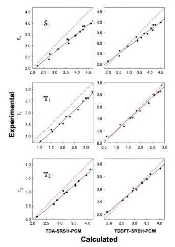
Fig. 4 Correlation plots of the calculated excitation energies (eV) vs. the experimental data for the training set molecules (Fig. 1). Red dashed lines of y = x lines represent the perfect fit for comparison.
