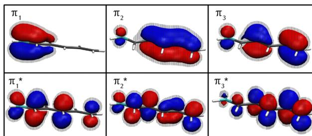
Fig. 2 Orbitals included in the active space for the SA(2)-CAS(6,6)SCF/6-31G electronic structure calculations. The  $S_1$ , with  $\pi\pi^*$  character, corresponds to an electron excited from orbital  $\pi_3$  to  $\pi_1^*$ .
