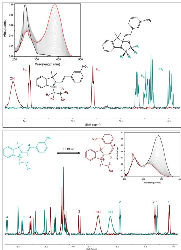
Fig. 3 Top: NMR spectrum of indolinoxazolidine 3 closed (blue) and ring-opened (red) forms following acidification, which is accompanied by an absorption band at 385 nm (inset). UV-Vis spectra were recorded every 0.5 s, with the photostationary state being reached in all cases after around 10 m. Bottom: *trans* (blue) and *cis* (red) forms with associated UV-Vis absorptions (inset) from initial (black) to final (red).
