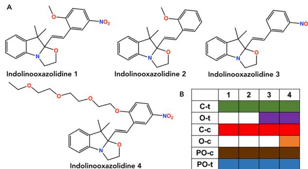
Fig. 4 a) The indolinoxazolidines studied. (b) The switching states accessible to the four indolinoxazolidines. C-t is closed-*trans* (where the oxazolidine ring is closed and the double bond is *trans*), O-t is open-*trans*, C-c is closed-*cis*, O-c is open-*cis*, PO-c is protonated open-*cis* (the oxazolidine ring is opened with acid), and PO-t is protonated open-*trans*.
