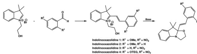
**Fig. 2** The synthesis of indolinoxazolidines. A functionalized aromatic aldehyde is condensed with an indolium bromide salt, which gives a salt of the ring-opened indolinoxazolidine. The salt is then ring-closed using an inorganic base to provide the final photoswitch. Here, triethylene glycol ethyl ether is shortened to TEG.
