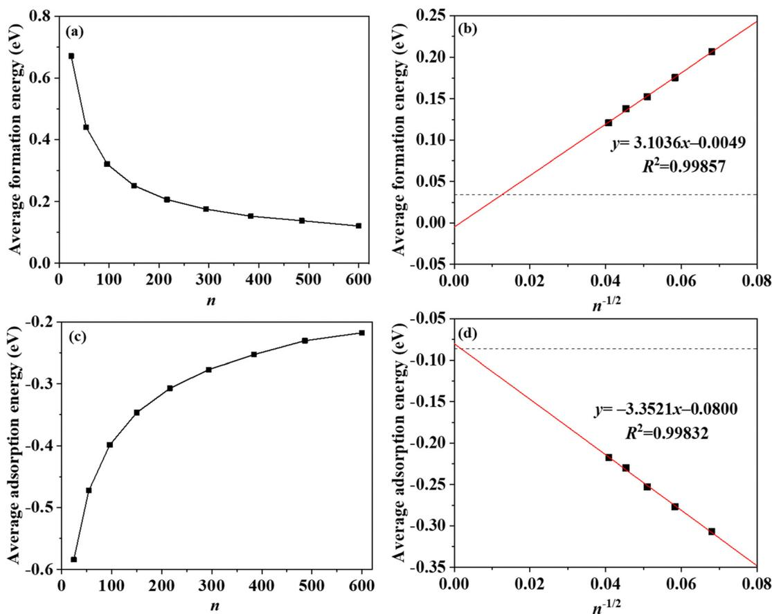
Fig. 7 Graphene nanosheets on the Cu(111) surface: relationship between average formation energy and the number of carbon atoms (a) and (b), as well as the relationship between average adsorption energy and the number of carbon atoms (c) and (d). The fitting method excludes data points with a small number of carbon atoms. The dashed lines represent the results of periodic graphene.
