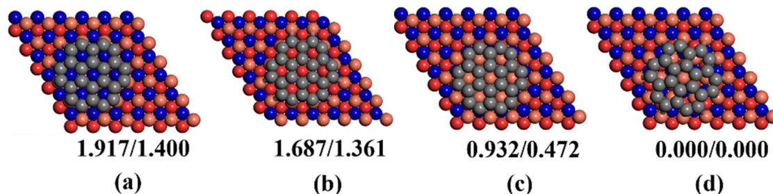
Fig. 4 Optimized graphene  $C_{24}$  structures on the Cu(111) surface with different adsorption sites: (a) the carbon atom occupying the TOP and FCC sites, (b) the carbon atom occupying the TOP and HCP sites, (c) the carbon atom occupying the HCP and FCC sites, (d) the most stable configuration of  $C_{24}$  on the Cu(111) surface. Relative energies of the lowest-energy structures calculated using HDNNP and DFT, with DFT results shown after the slash. All energies are given in units of eV.
