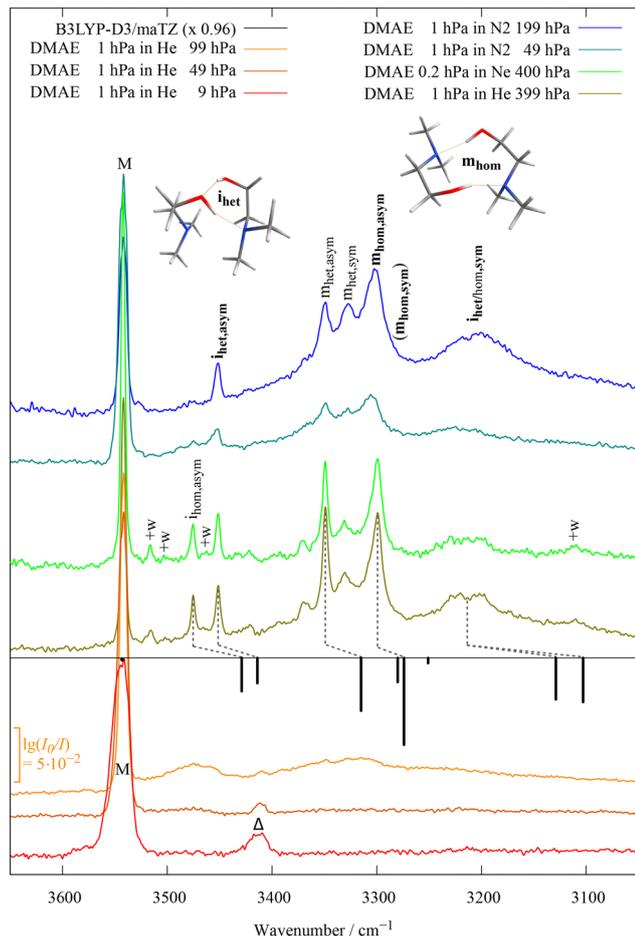
Fig. 7 IR spectra of dimethylaminoethanol (DMAE) for different expansion conditions with He (bottom), Ne (center) and  $N_2$  (top) as carrier gases and comparison with harmonic prediction for monomer and dimers (black). Assignments in bold refer to the more stable conformations of a given hydrogen bond topology. See text and ESI† for details.
