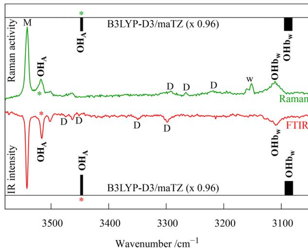
**Fig. 10** Comparison of Raman and (flipped) FTIR spectra of DMAE water co-expansions with  $0.96\times$  wavenumber-scaled harmonic predictions. Predicted relative intensities for the inserted 1:1 complex correspond to vertical bar areas (matched to the band intensities marked with a star). M, D and w mark DMAE monomer, dimer and water monomer transitions, respectively.
