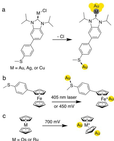
Fig. 9 (a) Schematic illustration of *in situ* electrochemical reduction of NHC–M–Cl complexes in forming C–M–Au bonds. (b) Formation of an Fe–Au bond in single-molecule junctions upon oxidation of ferrocene by a 405 nm laser or 450 mV applied voltage in an ionic solution. (c) Formation of oxidized ruthenocene and osmocene junctions in a polar solvent environment through Au–metal bonds on one end and an Au– $\pi$  interaction on the other.
