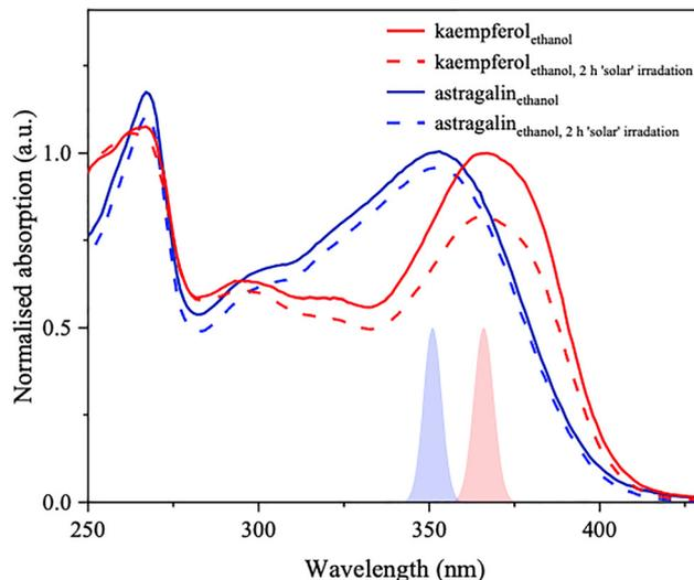
Fig. 2 UV-Visible absorption spectra of kaempferol (red) and astragalins (blue) in ethanol before and after 2 hours' 'solar' irradiation. Shaded plots are approximate profiles of the 'pump' pulses used in fs-TEAS for each solution.
