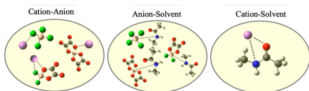
Fig. 2 Schematic of the interactions: cation-anion, anion-solvent, and cation-solvent.
