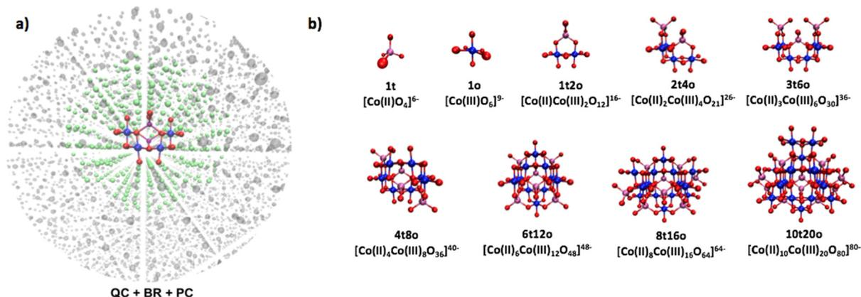
**Fig. 3** (a) Graphical representation of the embedded cluster approach for the  $\text{Co}_3\text{O}_4$  2t4o cluster. Color coding: QC region: Co(II) (purple); Co(III) (blue); O (red). BR/ECPs region: cECPs (green). PC region (grey). (b) Series of  $\text{Co}_3\text{O}_4$  models for QCs. Nomenclature 't' stands for tetrahedral ( $T_d - [\text{Co(II)}\text{O}_4]^{6-}$ ) and 'o' for distorted octahedral ( $D_{3d} - [\text{Co(III)}\text{O}_6]^{9-}$ ) substructures.
