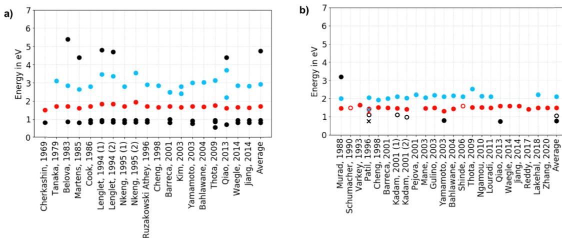
Fig. 1 Overview of experimental (a) absorption bands<sup>29,32–38,51–57,131–134</sup> and (b) band gaps<sup>26,29,31–50</sup> found in the literature. Red and blue symbols: the two most frequently reported band gap values – approx.  $1.51 \text{ eV}$  (red) and  $2.14 \text{ eV}$  (blue) – along with their associated absorption features. Black symbols: other reported absorption bands and band gaps. Filled circles: direct band gaps. Empty circles: indirect band gaps. Cross: forbidden gaps.
