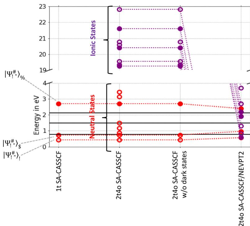
Fig. 6 First excited states of ligand field transitions in Al<sub>2</sub>CoO<sub>4</sub> with system size 1t as high spin ( $2S + 1 = 4$ ) and 2t4o computed for 'neutral' (red) and 'ionic' (purple) antiferromagnetic states ( $2S + 1 = 1$ ) with SA-CASSCF and SA-CASSCF/NEVPT2. Dark states (empty circle), 'potentially' non-dark states (half-filled circles), and non-dark states (filled circles).
