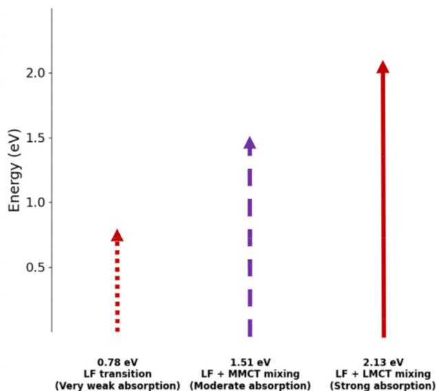
Fig. 9 Schematic representation of the optical transitions in  $\text{Co}_3\text{O}_4$ . Arrows indicate the observed transitions at 0.78 eV, 1.51 eV, and 2.13 eV corresponding to the experimentally observed band gaps. Red: dominantly 'neutral' states, purple: dominantly 'ionic' states. The lines qualitatively reflect oscillator strength: dotted corresponds to weaker, dashed to moderate, and solid lines to stronger absorption.
