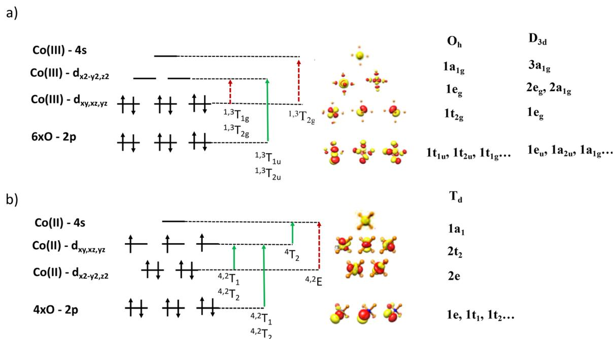
**Fig. 4** Schematic representation of excited states in (a)  $[\text{Co(III)}\text{O}_6]^{9-}$  ( $O_h/D_{3d}$ ) and (b)  $[\text{Co(II)}\text{O}_4]^{6-}$  ( $T_d$ ). Dotted red lines: electric dipole-forbidden transitions, solid green lines: electric dipole-allowed transitions. Lowercase and uppercase symmetry labels represent orbital and state symmetry labels, respectively.
