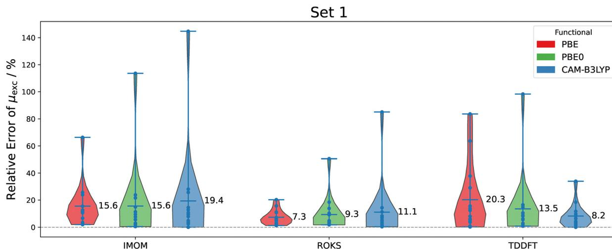
Fig. 4 Relative deviation (MAPD) of the excited-state dipole moments  $\mu_{\text{exc}}$  of set 1 from the TBE<sup>16</sup> reference.
