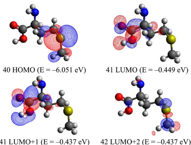
**Fig. 2** Some molecular orbitals of L-methionine calculated in the ground-state geometry.
