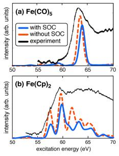
Fig. 10 XUV spectra of (a) Fe(CO)<sub>5</sub> and (b) Fe(Cp)<sub>2</sub> at the Fe M-edge, comparing CAM-B3LYP/CIS simulations to experimental spectra from ref. 130. Calculations employ the def2-TZVPD basis set with 200 singlet and 200 triplet states. Transition energies were broadened using a Lorentzian function (FWHM = 0.5 eV) but have not been shifted
