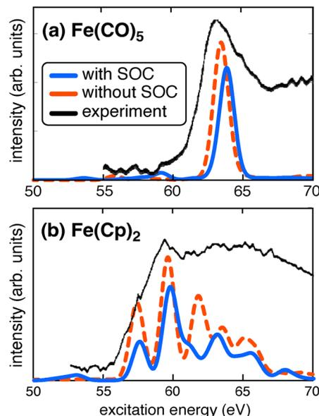
Fig. 10 XUV spectra of (a)  $\text{Fe}(\text{CO})_5$  and (b)  $\text{Fe}(\text{Cp})_2$  at the Fe M-edge, comparing CAM-B3LYP/CIS simulations to experimental spectra from ref. 130. Calculations employ the def2-TZVPD basis set with 200 singlet and 200 triplet states. Transition energies were broadened using a Lorentzian function (FWHM = 0.5 eV) but have not been shifted.
