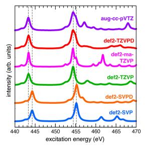
Fig. 2 Basis set effects on the Ti L<sub>2.3</sub>-edge spectrum of TiCl<sub>4</sub>, computed at the CAM-B3LYP/CIS + SOC level as described in Fig. 1. Spectra are normalized separately so that the main feature (around 455 eV) has the same intensity in each case. Vertical dashed lines are guides to the eye, aligned with the most intense L2 and L3 features at the top and at the bottom
