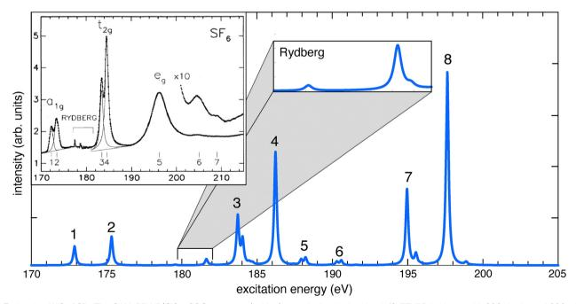
Fig. 7 L-edge XAS of SF<sub>6</sub>. The CAM-B3LYP/CIS + SOC spectrum (in blue) was obtained using the def2-TZVPD basis set with 200 singlet and 200 triplet states. Individual transition energies were shifted by 5 eV and broadened with a Lorentzian function (FWHM = 0.3 eV). The experimental spectrum (inset) is reproduced from ref. 134; copyright 1993 American Physical Society.
