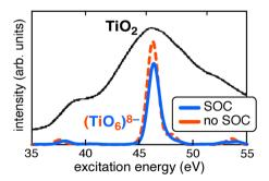
Fig. 11 XUV spectra at the Ti M-edge, for a rutile TiO<sub>2</sub> film (experiment) and its fundamental octahedral unit ( ${\rm TiO_6}$ )<sup>8-</sup> (CAM-B3LYP/CIS calculation). The experimental spectrum is reproduced from ref. 144 but was originally recorded in ref. 143. Calculations use the def2-TZVPD basis set and include 200 singlet and 200 triplet states, with transition energies that are broadened using a Lorentzian function (FWHM = 0.5 eV) but not shifted.
