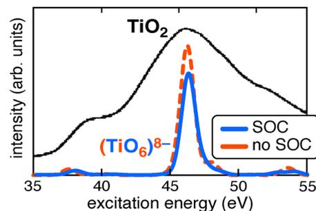
Fig. 11 XUV spectra at the Ti M-edge, for a rutile  $\text{TiO}_2$  film (experiment) and its fundamental octahedral unit  $(\text{TiO}_6)^{8-}$  (CAM-B3LYP/CIS calculation). The experimental spectrum is reproduced from ref. 144 but was originally recorded in ref. 143. Calculations use the def2-TZVPD basis set and include 200 singlet and 200 triplet states, with transition energies that are broadened using a Lorentzian function (FWHM = 0.5 eV) but not shifted.
