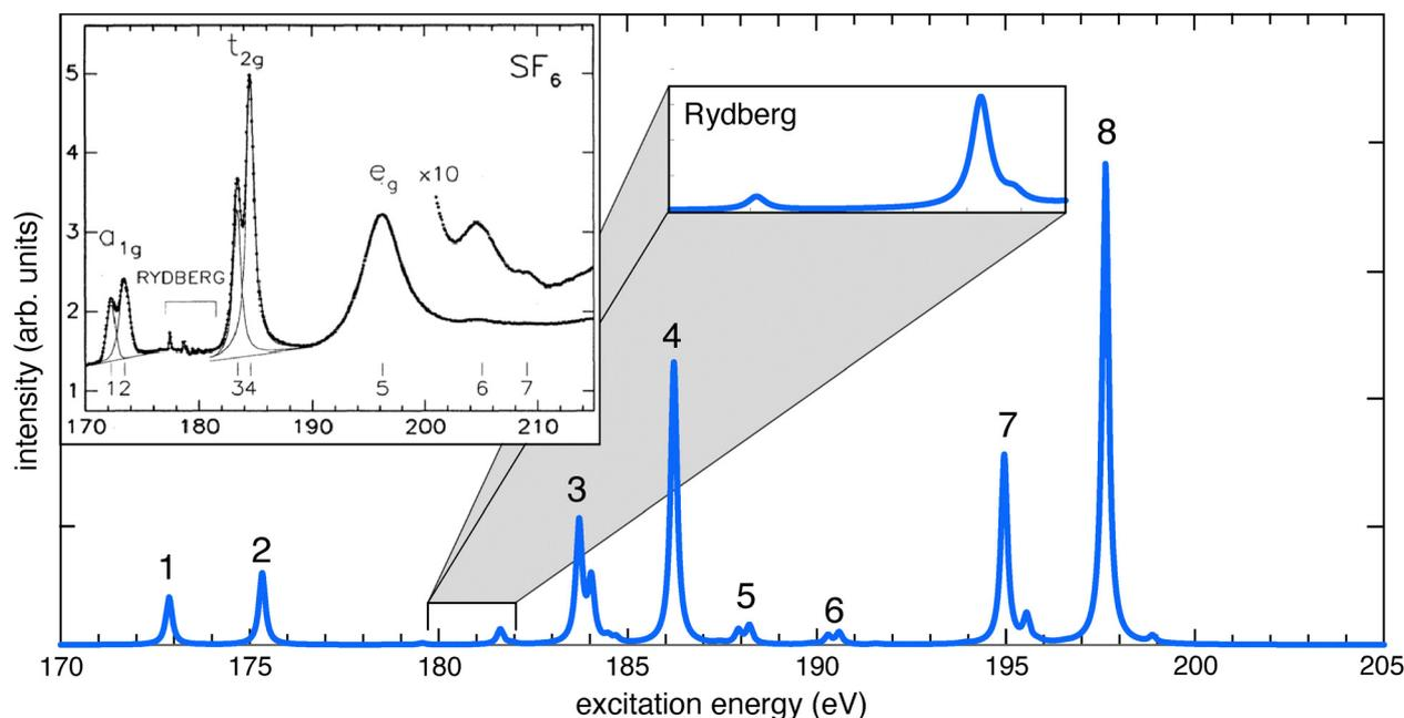
Fig. 7 L-edge XAS of  $SF_6$ . The CAM-B3LYP/CIS + SOC spectrum (in blue) was obtained using the def2-TZVPD basis set with 200 singlet and 200 triplet states. Individual transition energies were shifted by 5 eV and broadened with a Lorentzian function (FWHM = 0.3 eV). The experimental spectrum (inset) is reproduced from ref. 134; copyright 1993 American Physical Society.
