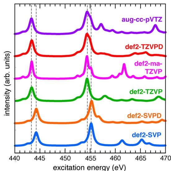
Fig. 2 Basis set effects on the Ti  $L_{2,3}$ -edge spectrum of  $\text{TiCl}_4$ , computed at the CAM-B3LYP/CIS + SOC level as described in Fig. 1. Spectra are normalized separately so that the main feature (around 455 eV) has the same intensity in each case. Vertical dashed lines are guides to the eye, aligned with the most intense  $L_2$  and  $L_3$  features at the top and at the bottom.
