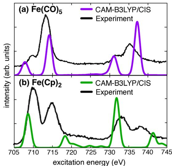
Fig. 9  $L_{2,3}$ -edge spectra of (a)  $\text{Fe}(\text{CO})_5$  and (b)  $\text{Fe}(\text{Cp})_2$ , comparing experiment (with an offset baseline) to CAM-B3LYP/CIS + SOC simulations. The calculations employ the def2-TZVPD basis set with 200 singlet and 200 triplet states, broadened using a Lorentzian function (FWHM = 0.7 eV). The computed spectra were shifted by (a) 8.0 eV and (b) 10.0 eV in order to align with experimental spectra that are reproduced from ref. 130.
