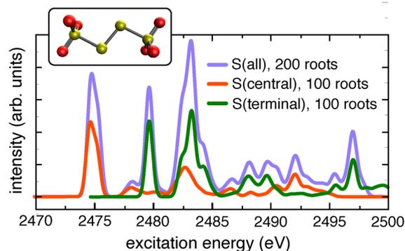
Fig. 5 XAS of (S<sub>4</sub>O<sub>6</sub>)<sup>2-</sup> at the sulfur K-edge, illustrating how calculations with different active spaces can be used to assign spectral features. Spectra were computed using CAM-B3LYP/CIS + SOC with the def2-TZVPD basis set and Lorentzian broadening (FWHM = 0.3 eV). CVS active spaces contain S(1s) orbitals on the atoms indicated in the legend.
