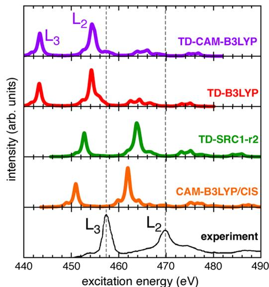
Fig. 1 Direct relation between the accuracy of TD-DFT calculations and the fraction of exact exchange, for Ti  $L_{2,3}$ -edge spectra of  $\text{TiCl}_4$ . Shown are four different TD-DFT approaches along with CAM-B3LYP/CIS, in comparison to an experimental spectrum from ref. 121. All calculations used the def2-TZVPD basis set and include 200 singlet and 200 triplet basis states. Individual transitions were broadened using a Lorentzian function with FWHM = 0.3 eV.
