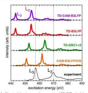
Fig. 1 Direct relation between the accuracy of TD-DFT calculations and the fraction of exact exchange, for Ti L<sub>2,3</sub>-edge spectra of TiCl<sub>4</sub>. Shown are four different TD-DFT approaches along with CAM-B3LYP/CIS, in comparison to an experimental spectrum from ref. 121. All calculations used the def2-TZVPD basis set and include 200 singlet and 200 triplet basis states. Individual transitions were broadened using a Lorentzian function with FWHM = 0.3 eV.
