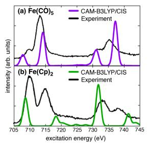
Fig. 9 L<sub>2.3</sub>-edge spectra of (a) Fe(CO)<sub>5</sub> and (b) Fe(Cp)<sub>2</sub>, comparing experiment (with an offset baseline) to CAM-B3LYP/CIS + SOC simulations. The calculations employ the def2-TZVPD basis set with 200 singlet and 200 triplet states, broadened using a Lorentzian function (FWHM = 0.7 eV). The computed spectra are were shifted by (a) 8.0 eV and (b) 10.0 eV in order to align with experimental spectra that are reproduced from ref. 130.
