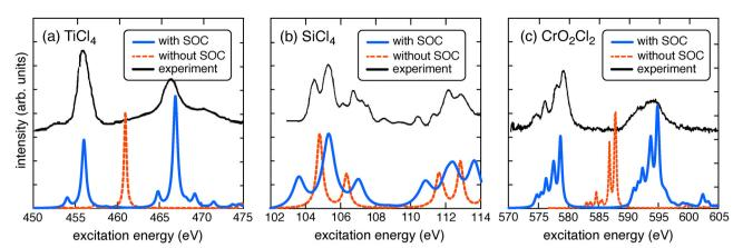
Fig. 3 Experimental  $L_{2.3}$ -edge spectra for (a) Ti in  $TiCl_4$ , <sup>121</sup> (b) Si in  $SiCl_4$ , <sup>126</sup> and (c) Cr in  $CrO_2Cl_2$ , <sup>127</sup> in comparison to CAM-B3LYP/CIS + SOC calculations. The latter employ the def2-TZVPD basis set with 200 singlet and 200 triplet excited states. Calculated transition energies were broadened using a Lorentzian function (FWHM = 0.3 eV) and shifted by (a) 5.0 eV, (b) 3.2 eV, and (c) 4.8 eV.
