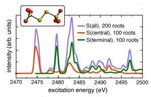
Fig. 5 XAS of  $(S_4O_6)^{2-}$  at the sulfur K-edge, illustrating how calculations with different active spaces can be used to assign spectral features. Spectra were computed using CAM-B3LYP/CIS + SOC with the def2-TZVPD basis set and Lorentzian broadening (FWHM = 0.3 eV). CVS active spaces contain S(1s) orbitals on the atoms indicated in the legend
