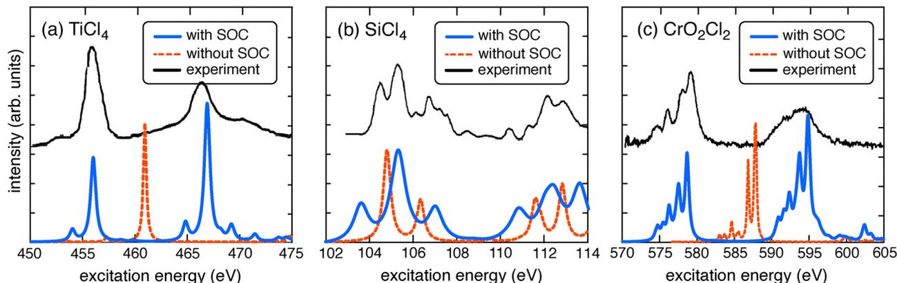
Fig. 3 Experimental  $L_{2,3}$ -edge spectra for (a) Ti in  $\text{TiCl}_4$ ,<sup>121</sup> (b) Si in  $\text{SiCl}_4$ ,<sup>126</sup> and (c) Cr in  $\text{CrO}_2\text{Cl}_2$ ,<sup>127</sup> in comparison to CAM-B3LYP/CIS + SOC calculations. The latter employ the def2-TZVPD basis set with 200 singlet and 200 triplet excited states. Calculated transition energies were broadened using a Lorentzian function (FWHM = 0.3 eV) and shifted by (a) 5.0 eV, (b) 3.2 eV, and (c) 4.8 eV.
