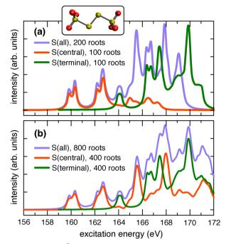
Fig. 6 XAS of  $(S_4O_6)^{2-}$  at the sulfur L-edge. All calculations were performed using CAM-B3LYP/CIS + SOC with def2-TZVPD, computing either (a) 200 or (b) 800 singlet and triplet excited states, which were then broadened using a Lorentzian function (FWHM = 0.2 eV). Spectra labeled S(terminal) and S(central) employ only the S(2p) orbitals on the indicated atoms, with a correspondingly smaller number of excited states, whereas S(all) uses all of the S(2p) orbitals.
