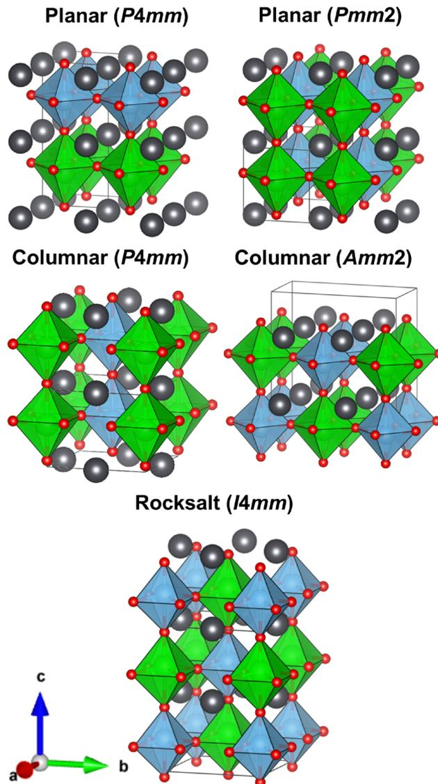
Fig. 1 Illustration of the optimized structures of the five different ordered  $\text{Pb}[\text{Zr}_{0.5}\text{Ti}_{0.5}]\text{O}_3$  models used in this work. Ti and its octahedra in blue, Zr and its octahedra in green, O in red, and Pb in grey. All structures are viewed from the same direction. Visualization made with the VESTA software.<sup>63</sup>
