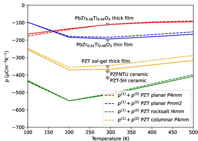
Fig. 6 Calculated pyroelectric coefficients for planar  $P4mm$  (red), planar  $Pmm2$  (blue), columnar  $P4mm$  (yellow) and rocksalt  $I4mm$  (green) orderings. Primary coefficient  $p^{(1)}$  in solid lines and total  $p$  ( $p^{(1)} + p^{(2)}$ ) in dashed lines. Experimental data in diamonds for PZT-5H<sup>76</sup> and PZFTU<sup>77</sup> ceramics, and with crosses for thin film,<sup>19</sup> sol-gel thick film,<sup>75</sup> and thick film.<sup>73</sup>
