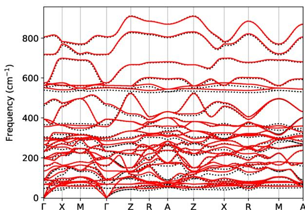
**Fig. 2** Anharmonic 300 K (red, solid) and harmonic (black, dotted) phonon dispersion of columnar  $P4mm$  PZT. Phonon dispersions of other ordered models are included in the (ESI<sup>†</sup>).
