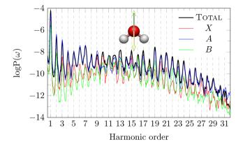
Fig. 4 Total and partial HHG spectra of H2O, with pulse polarisation parallel to the principal axis (z axis). This system corresponds to the configuration (c) of Fig. 2. The yellow double arrow represents the pulse polarisation, while a green arrow represents the direction of detection of the HHG signal.
