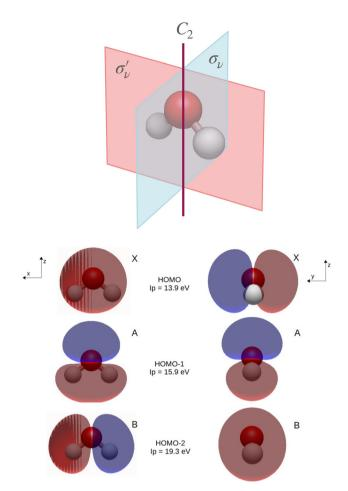
Fig. 1 Representation of the H<sub>2</sub>O molecule with  $\sigma_{\nu}$  and  $\sigma'_{\nu}$  reflection planes and the  $C_2$  rotational axis, and  $H_2O$  HF occupied MOs studied in this work
