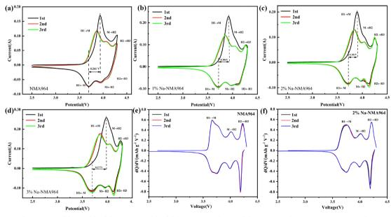
Fig. 4 Initial three CV curves of (a) NMA964, (b) 1%Na-NMA964, (c) 2%Na-NMA964, and (d) 3%Na-NMA964 with a scan rate of 0.2 mV s<sup>-1</sup>. The dQ/dVprofiles of the initial three cycles for (e) NMA964 and (f) 2%Na-NMA964.
