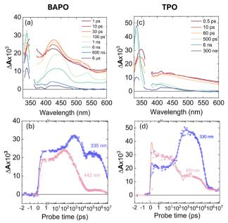
Fig. 4 TA spectra (top row) and selected kinetic traces (bottom row) obtained after excitation with 360 nm pulses (fs-ns) or 355 nm (ns-μs), of solutions of BAPO (a and b) and TPO (c and d), respectively. The spectra were merged at a delay of 6 ns.
