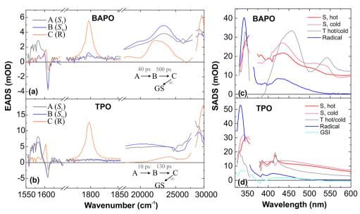
Fig. 9 Evolution-associated difference absorption spectra (EADS) and time constants obtained from a global analysis of the (a) BAPO and (b) TPO TRIR-UV/Vis data. The panels (c) and (d) show the SADS of femtosecond-microsecond UV/Vis BAPO and TPO TA data obtained by assuming the model in Fig. 10. The TRIR spectra in panel (a) and (b) were scaled to match their intensities with UV/Vis TA spectra.
