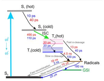
Reaction scheme, summarizing the mechanisms and their timescales in BAPO (red) and TPO (blue). The GSI component represents a small fraction of the TPO photoproduct, detectable on a microsecond
