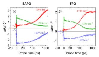
Fig. 7 Kinetic traces corresponding to the bleach of the parent compound (1609 cm<sup>-1</sup>, blue), the transient associated with the S<sub>1</sub> state (1585 cm<sup>-1</sup>, green), and the transient of the photoproduct mesitoyl radical band (1798 cm<sup>-1</sup>, red), obtained from the TRIR data of BAPO (a) and TPO (b) upon photoexcitation at 400 nm. Symbols indicate measured data, and solid lines indicate the results from the global fits.
