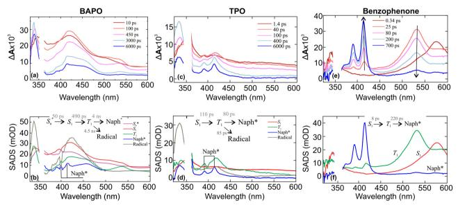
Fig. 8 (a), (c) and (e) TA spectra of BAPO, TPO and benzophenone 2-propanol solutions, containing naphthalene and (b), (d) and (f) SADS, obtained from global analysis. The empty region in spectra indicate area omitted due to the scattering of the pump pulse. The concentrations of BAPO, TPO and naphthalene were 3 mM, 6 mM and 300 mM, respectively
