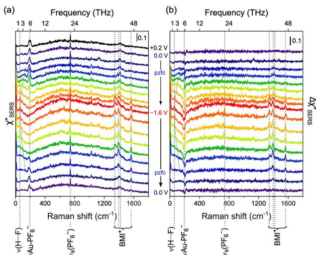
Fig. 3 (a) A series of SERS spectra in the reduced DOS format ( $\chi''_{\text{SERS}}$ ) for dry [BMI]PF<sub>6</sub>, measured on the Au surface under a potential cycle between  $0.0$  and  $-1.6$  V vs. Fc/Fc<sup>+</sup>. (b) Difference spectra of (a) with respect to the SERS spectrum taken at  $+0.2$  V.
