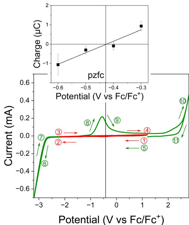
Fig. 1 Cyclic voltammograms of dry [BMI]PF<sub>6</sub> in capacitive (red) and faradaic (green) regions, measured on an Au electrode with a scan rate of 50 mV s<sup>-1</sup>. The numbers indicated show the order of the continuous potential cycles. The inset shows that the potential of zero free charge (pzfc) obtained using the immersion method is around -0.43 V.
