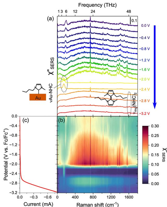
Fig. 6 (a) A series of SERS spectra in the reduced DOS format ( $\chi''_{\text{SERS}}$ ) for dry [BMI]PF<sub>6</sub>, measured under negative-going potential scan from 0.0 to -3.2 V vs. Fc/Fc<sup>+</sup>. (b) 2D contour plot of (a). (c) Linear sweep voltammogram of dry [BMI]PF<sub>6</sub> measured on the SERS-active Au electrode with a scan rate of 50 mV s<sup>-1</sup>.
