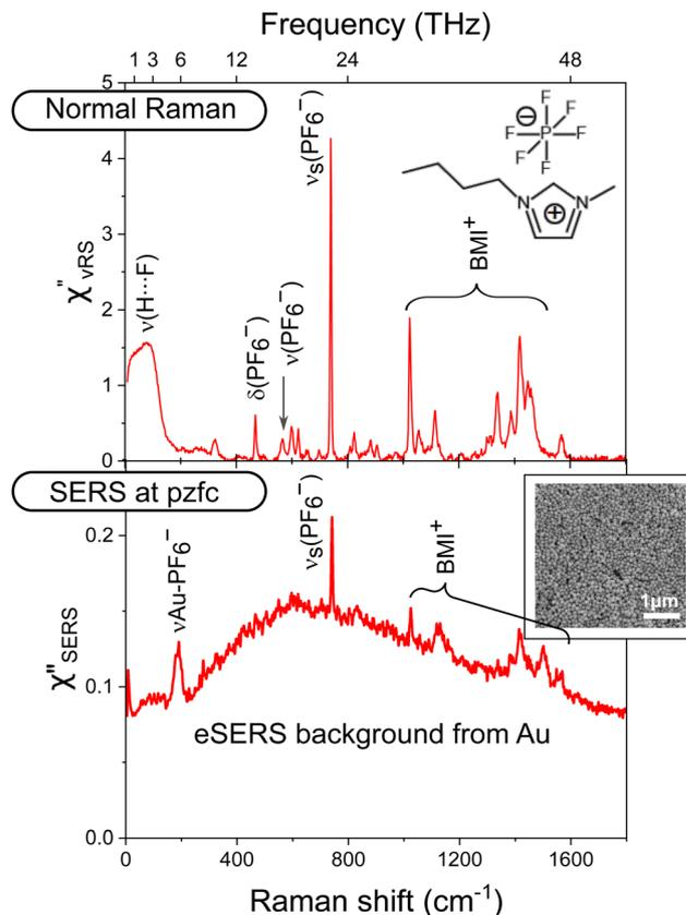
Fig. 2 (Top panel) Normal vibrational Raman spectrum in the reduced DOS format ( $\chi''_{\text{vRS}}$ ) for the bulk solution of dry [BMI]PF<sub>6</sub> (water impurity of less than 5 ppm), measured at 632.8 nm. (Bottom panel) SERS spectrum in the reduced DOS format ( $\chi''_{\text{SERS}}$ ) for dry [BMI]PF<sub>6</sub> on the Au electrode, measured at pzfc using 632.8 nm excitation. The inset shows a SEM image of the SERS-active Au surface.
