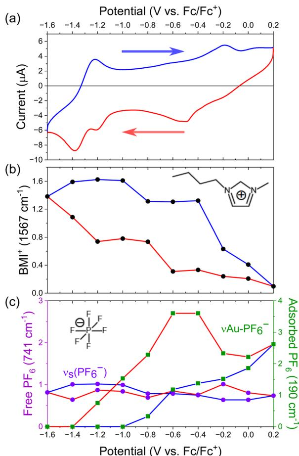
Fig. 5 (a) A cyclic voltammogram of dry [BMI]PF<sub>6</sub>, measured on the SERS-active Au electrode with a scan rate of 50 mV s<sup>-1</sup>. (b) Potential dependence of νSERS intensity of BMI-cations at 1567 cm<sup>-1</sup>. (c) Potential dependence of νSERS intensities of PF<sub>6</sub><sup>-</sup>-anions at 741 cm<sup>-1</sup> and 190 cm<sup>-1</sup>.
