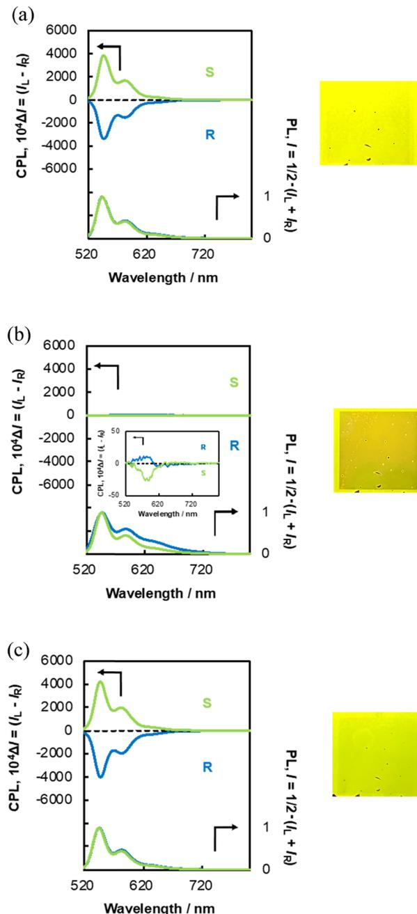
**Fig. 4** CPL (upper chart) and PL spectra (lower chart) of  $N^*$ -LC-6CB/(*R,R*)-**CPDI** (blue) and  $N^*$ -LC-6CB/(*S,S*)-**CPDI** (green) and luminescent images of  $N^*$ -LC-6CB/(*S,S*)-**CPDI** (right-hand images) acquired (a) before voltage application at 0 V, (b) at 30 V, and (c) after voltage application at 0 V. The CPL and PL spectra were acquired at an excitation wavelength of 480 nm, while the luminescent images were acquired at an excitation wavelength of 365 nm.
