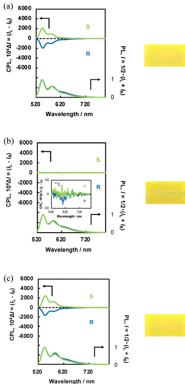
Fig. 8 CPL (upper chart) and PL spectra (lower chart) of the nematic liquid crystal states of N\*-LC-6CB/(R,R)-BPP (blue) and N\*-LC-6CB/(S,S)-BPP (green) and luminescent images of N\*-LC-6CB/(S,S)-BPP (right-hand images) acquired at (a) 25 °C before heating, (b) 40 °C, and (c) 25 °C after heating. The CPL and PL spectra were acquired at an excitation wavelength of 480 nm, while the luminescent images were acquired at an excitation wavelength of 365 nm.
