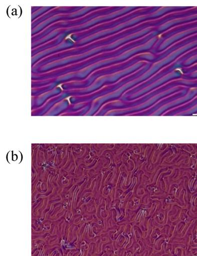
Fig. 2 Polarised optical microscopy (POM) images of (a) N<sup>\*</sup>-LC-6CB/(*S,S*)-**BPP** and (b) N<sup>\*</sup>-LC-6CB/(*S,S*)-**CPDI**.
