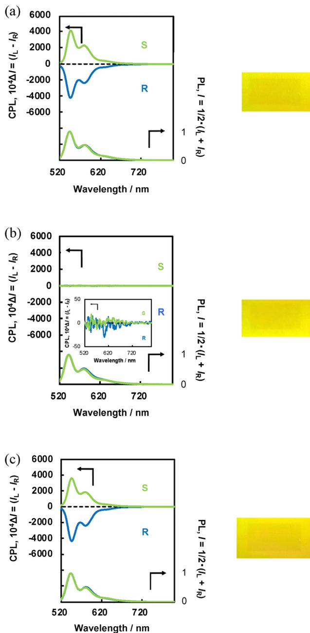
Fig. 9 CPL (upper chart) and PL spectra (lower chart) of the nematic liquid crystal states of N\*-LC-6CB/(R,R)-CPDI (blue) and N\*-LC-6CB/(S,S)-CPDI (green) and luminescent images of N\*-LC-6CB/(S,S)-CPDI (right-hand images) acquired at (a) 25 °C before heating, (b) 40 °C, and (c) 25 °C after heating. The CPL and PL spectra were acquired at an excitation wavelength of 480 nm, while the luminescent images were acquired at an excitation wavelength of 365 nm.
