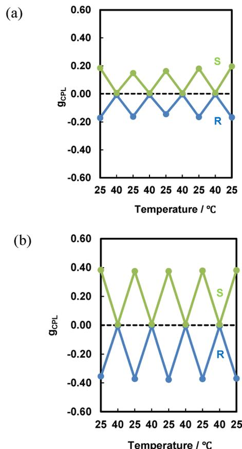
Fig. 10 Evolution of the  $g_{\text{CPL}}$  of (a) N\*-LC-6CB/(R,R)-BPP (blue) and N\*-LC-6CB/(S,S)-BPP (green) and (b) N\*-LC-6CB/(R,R)-CPDI (blue) and N\*-LC-6CB/(S,S)-CPDI (green) upon switching between 25 and 40 °C. An excitation wavelength of 480 nm was used for CPL and PL.
