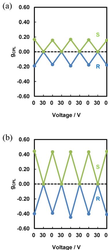
Fig. 6 Evolution of the  $g_{\text{CPL}}$  of (a) N\*-LC-6CB/(R,R)-BPP (blue) and N\*-LC-6CB/(S,S)-BPP (green) and (b) N\*-LC-6CB/(R,R)-CPDI (blue) and N\*-LC-6CB/(S,S)-CPDI (green) upon switching between 0 and 30 V. An excitation wavelength of 480 nm was used for CPL and PL.
