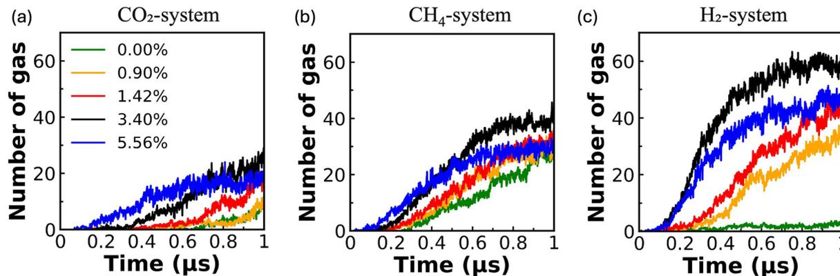
Fig. 6 The number of gas molecules encapsulated within the hydrate cages as a function of time at different THF concentrations for (a) the CO<sub>2</sub> system, (b) the CH<sub>4</sub> system, and (c) the H<sub>2</sub> system.
