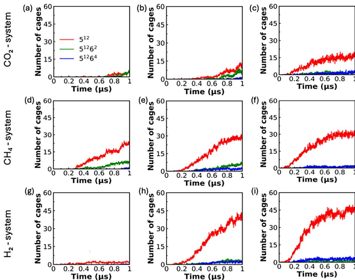
Fig. 4 Time evolution of the number of hydrate cages –  $5^{12}$ ,  $5^{12}6^2$ , and  $5^{12}6^4$  – formed in (a)–(c) the CO<sub>2</sub> system, (d)–(f) the CH<sub>4</sub> system, and (g)–(i) the H<sub>2</sub> system at THF concentrations of 0% (left panels), 1.42% (middle panels), and 5.56% (right panels).
