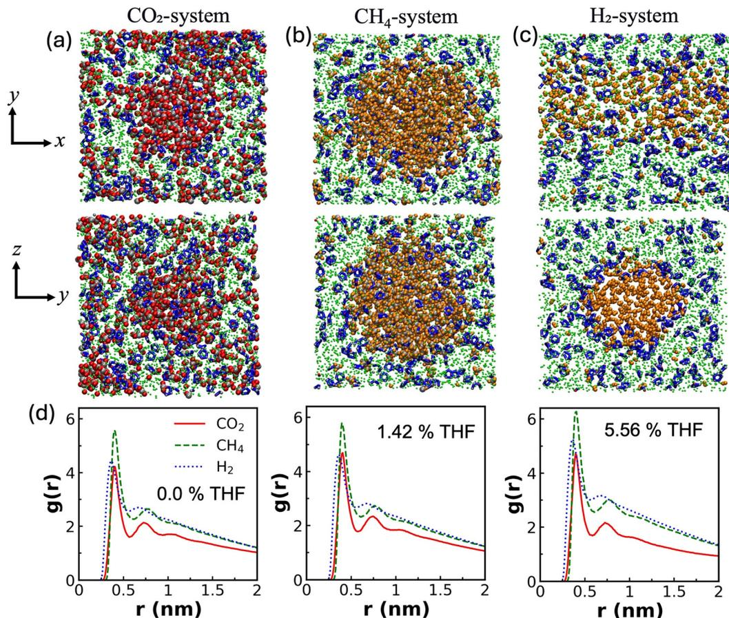
Fig. 2 Side views of MD snapshots captured at the end of 5 ns of initial equilibration at 300 K and 10 MPa in the presence of 5.56 mol% THF for gas systems: (a) CO<sub>2</sub>, (b) CH<sub>4</sub>, and (c) H<sub>2</sub>. Atom colors are the same as those denoted in Fig. 1. Panel (d) shows the radial distribution function of gas molecules computed over the 5–10 ns interval at 300 K and 10 MPa for THF concentrations of 0 (left), 1.42 (middle), and 5.56% (right).
