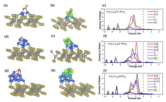
Fig. 3 The most stable adsorption configurations, the isosurface of the charge density difference with an isovalue of  $0.003 \, \text{Å}^{-1}$ , and the PDOS for CO<sub>2</sub> on Cu<sub>3</sub>@WTe<sub>2</sub>: (a)-(c), Cu<sub>8</sub>@WTe<sub>2</sub> (d)-(f) and Cu<sub>13</sub>@WTe<sub>2</sub> (g)-(i). The blue (yellow) wireframes denote the loss (gain) of electrons with the isosurface values set as  $0.003 \text{ Å}^{-3}$ . The Fermi level is assigned at 0 eV.
