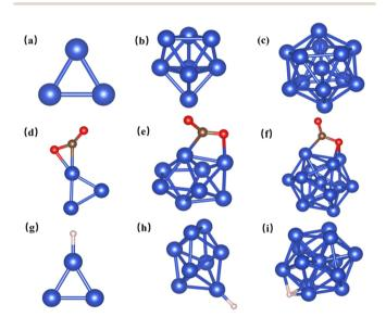
Fig. 1 (a)–(c) Structures of the pristine  $Cu_3$ ,  $Cu_8$  and  $Cu_{13}$  clusters. (d)–(f) The most stable adsorption configurations for CO<sub>2</sub> on Cu<sub>3</sub>, Cu<sub>8</sub>, and Cu<sub>13</sub> clusters. (g)-(i) The optimized configurations for H adsorption on Cu<sub>3</sub>, Cu<sub>8</sub>, and Cu<sub>13</sub>.
