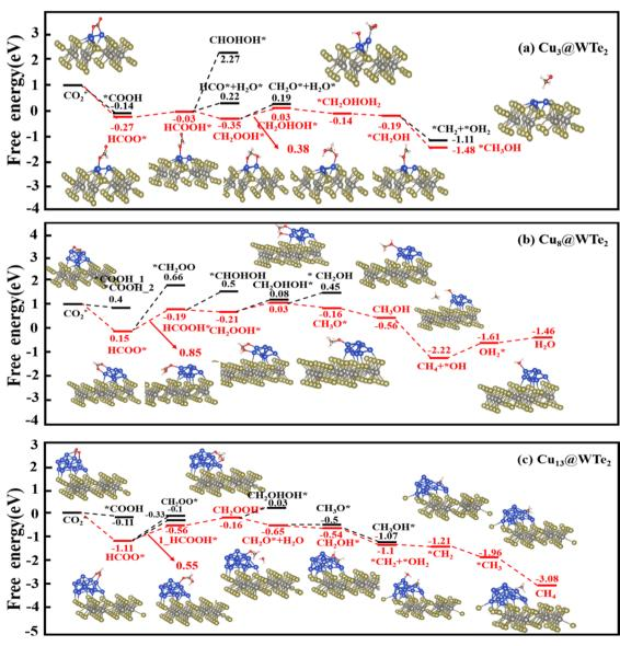
Fig. 4 Free energy diagram for the electrochemical CO<sub>2</sub>RR on (a) Cu<sub>3</sub>@WTe<sub>2</sub>, (b) Cu<sub>8</sub>@WTe<sub>2</sub>, and (c) Cu<sub>13</sub>@WTe<sub>2</sub>.
