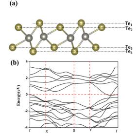
Fig. 2 (a) Schematic of the  $3 \times 2$  supercell of T'-WTe<sub>2</sub>. W and Te atoms are denoted by grey and orange spheres, respectively. (b) Band structure for the T'-WTe2 monolayer.
