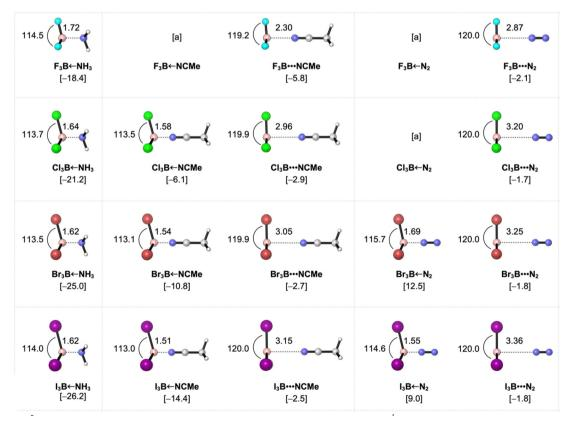
Fig. 2 Geometries (in Å, deg.) and the electronic bond energies  $\Delta E$  in brackets (in kcal mol<sup>-1</sup>) of the  $X_3B-LB$  Lewis pairs ( $X_3=F_3$ ,  $Cl_3$ ,  $Br_3$ ,  $I_3$ ;  $LB=NH_3$ , MeCN,  $N_2$ ) in  $C_{3v}$  symmetry, computed at ZORA-BLYP-D3(BJ)/TZ2P. <sup>a</sup> Lewis adduct does not exist.
