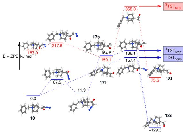
Fig. 12 Potential energy surface of the  $N_2$ -loss reaction of benzyl quinuclidinium  $\alpha$ -diazo ketone **10** via the respective carbenes **17s/17t** in either a stepwise or a concerted Wolff rearrangement reaction to the singlet ketene **18**. All optimisations, energies, and frequencies calculated using B3LYP-D3(BJ)//cc-pVTZ.
