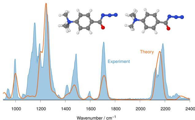
Fig. 2 IRIS spectrum of the aromatic acyl azide precursor **7** at  $m/z$  205 (blue shadowed trace) compared with the weighted average spectrum of isomer 1 (0.0 kJ mol<sup>-1</sup>) and isomer 2 (0.2 kJ mol<sup>-1</sup>) orange trace (anharmonic computations, traces (b) and (c) in Fig. 1). Scaling of below 2000 cm<sup>-1</sup>: 0.99. Scaling above 2000 cm<sup>-1</sup>: 0.955.
