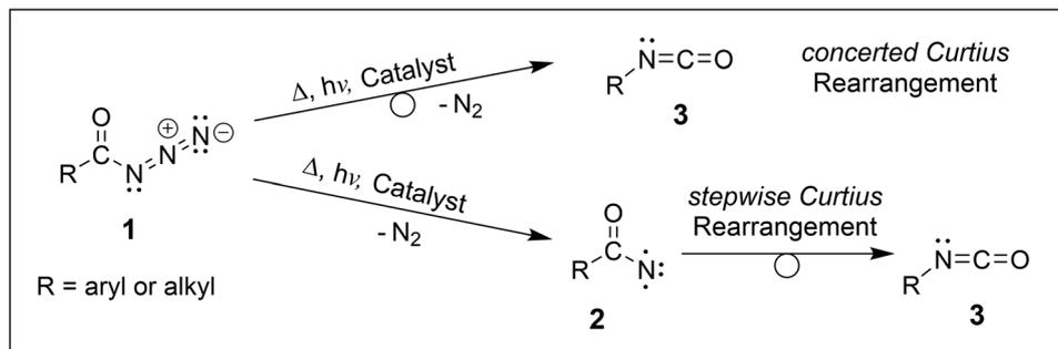
**Scheme 1** The Curtius rearrangement reaction of acyl azides **1** leads to the  $N_2$  release upon activation and ultimately yields isocyanates **3** either *via* acyl nitrene intermediates **2** (shown here in the triplet electronic state with two unpaired electrons) in a stepwise reaction or along a direct concerted reaction pathway.<sup>3</sup>
