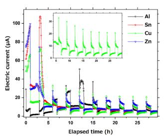
Fig. 9 Time-dependence of electric current in gel columns (L = 50 mm,  $\phi$  = 4 mm,  $C_{\rm se}$  = 10 mM) using Al, Sn, Cu, and Zn anodes at 298 K under the following voltage conditions:  $E_{\rm H}$  = 3 V,  $E_{\rm L}$  = 1 V,  $T_{\rm H}$  = 1 h,  $T_{\rm L}$  = 2 h, and  $N_{\rm C}$  = 10. Each system had a Cu cathode. Inset: Enlarged plot for system
