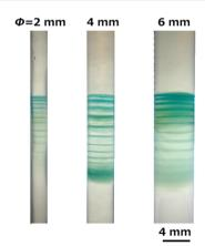
Fig. 6 Banding patterns of  $Cu(OH)_2$  precipitates formed in gel columns with different diameters (L=50 mm,  $\phi=2$ , 4, and 6 mm,  $C_{se}=10$  mM) through RTR processes at 298 K under the following voltage conditions:  $E_{H}=3$  V,  $E_{L}=1$  V,  $T_{H}=1$  h,  $T_{L}=2$  h, and  $N_{C}=16$ . Each system had a Cu anode and Cu cathode.
