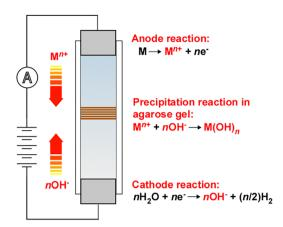
Fig. 1 Schematic of the basic RTR system with agarose gel inserted between two metal rods in a plastic tube. The applied voltage is switched between high voltage  $E_{\rm H}$  and low voltage  $E_{\rm L}$  for times  $T_{\rm H}$  and  $T_{\rm L}$ , respectively, for  $N_C$  cycles. The arrows indicate the direction of the movement of the reactant ions in the electric field.
