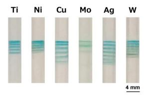
Fig. 3 Banding patterns of  $Cu(OH)_2$  precipitates in gel columns (L =50 mm,  $\phi$  = 4 mm,  $C_{\text{se}}$  = 10 mM) through RTR processes using Ti, Ni, Cu, Mo, Ag, and W cathodes at 298 K under the following voltage conditions:  $E_H = 3 \text{ V}$ ,  $E_L = 1 \text{ V}$ ,  $T_H = 1 \text{ h}$ ,  $T_L = 2 \text{ h}$ , and  $N_C = 8$ . Each system had a Cu anode.
