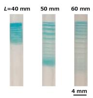
**Fig. 5** Banding patterns of Cu(OH)<sub>2</sub> precipitates in gel columns with different lengths (L=40, 50, and 60 mm,  $\phi=4$  mm,  $C_{\rm se}=10$  mM) through RTR processes at 298 K under the following voltage conditions:  $E_{\rm H}=3$  V,  $E_{\rm L}=1$  V,  $T_{\rm H}=1$  h,  $T_{\rm L}=2$  h, and  $N_{\rm C}=15$ . Each system had a Cu anode and Cu cathode.
