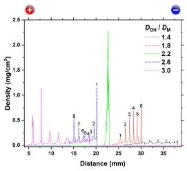
Fig. 11 Calculated  $D_{OH}/D_{M}$  dependence of the precipitate density distributions at t = 24 h ( $N_C = 8$ ) for  $f_i = 1.0$ . For the data of  $D_{OH}/D_M = 1.8$  and 2.6. the precipitation bands are numbered according to the order in which they are generated. The sides of the anode (+) and cathode (-), which exist at distances of 0 and 50 mm, respectively, are indicated at the top of the
