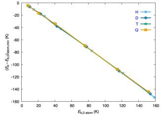
Fig. 7 Change in the kinetic energy of the atom at the dynamical minimum, as a function of the initial kinetic energy of the atom,  $E_{k,0}$ , for the four isotopic variants (H, D, T and Q). In some cases there are more than a single minimum (see the text).
