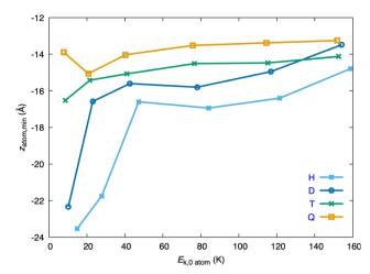
Fig. 8 Z-coordinate of the atom at the dynamical minimum,  $z_{Xm}$ , as a function of the initial kinetic energy of the atom,  $E_{k,0}$ , for the four isotopic variants (H, D, T and Q). In some cases there are more than a single minimum (see the text).
