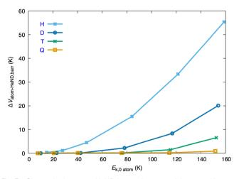
**Fig. 3** Change in the atom–HeND interaction potential energy,  $V_{\rm X-HeND}$ , at the dynamical barrier, as a function of the initial kinetic energy of the atom,  $E_{\rm k,0}$ , for the four isotopic variants (H, D, T and Q). Changes are relative to the initial reactant state.
