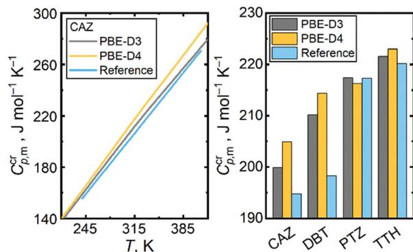
Fig. 6 Illustration of the temperature trends of experimental isobaric heat capacities  $C_{p,m}^{cr}$  for crystalline carbazole and those calculated using the quasi-harmonic protocol and PBE-D3 and PBE-D4 models (left); and a comparison of experimental and calculated crystal-phase heat capacities at 298.15 K and ambient pressure for all the target materials (right).
