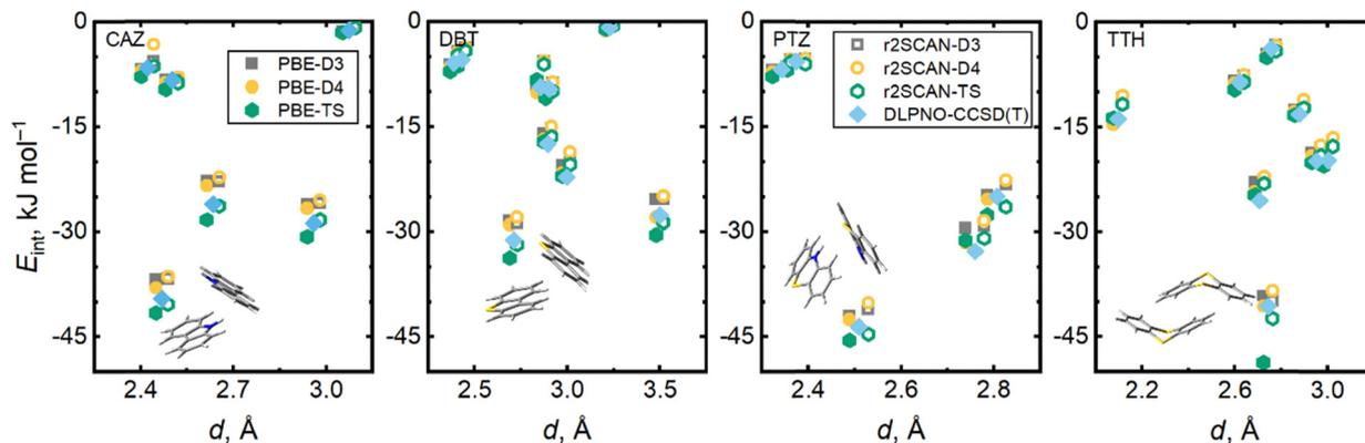
Fig. 8 Comparison of the closest pair interactions extracted from the target crystal structures calculated using either PBE or  $r^2$ SCAN functional and either D3, D4 or TS dispersion corrections with the reference results of DLPNO-CCSD(T)/CBS calculations. Geometries of the dimers corresponding to the strongest attractive interaction in individual crystal structures are depicted as insets.
