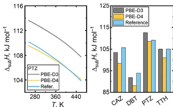
Fig. 7 Illustration of the temperature trends of experimental sublimation enthalpy for crystalline phenothiazine and those calculated using the quasi-harmonic protocol and PBE-D3 and PBE-D4 models (left); and a comparison of experimental and calculated sublimation enthalpies at 298.15 K for all the target materials (right).
