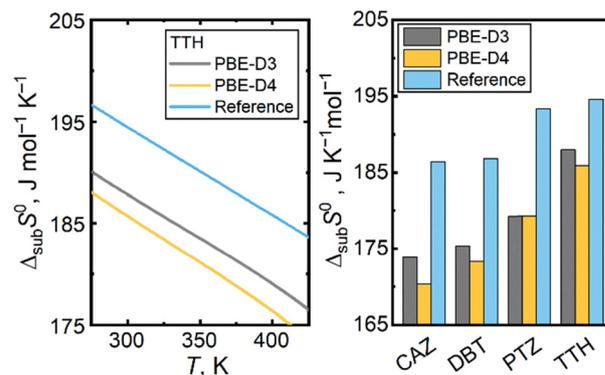
Fig. 10 Illustration of the temperature trends of experimental standard sublimation entropy for crystalline thianthrene and those calculated using the quasi-harmonic protocol and PBE-D3 and PBE-D4 models (left); and a comparison of experimental and calculated standard sublimation entropies at 298.15 K and 100 kPa for all the target materials (right).
