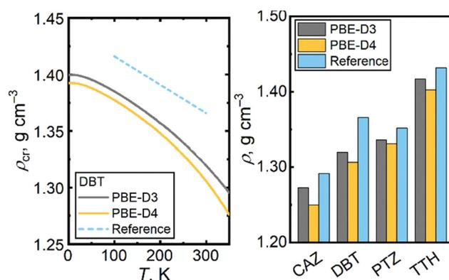
Fig. 5 Illustration of trends of experimental reference densities  $\rho$  for dibenzothiophene and those calculated using the quasi-harmonic protocol and PBE-D3 and PBE-D4 models (left); and a comparison of experimental and calculated crystal-phase densities at 298.15 K and at the standard pressure for all the target materials (right).
