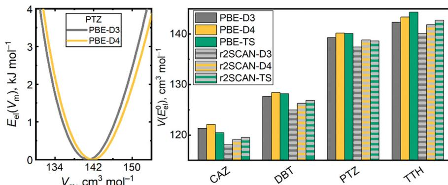
Fig. 3 Illustration of how static electronic energies  $E_{el}$  modelled by PBE-D3 and PBE-D4 for phenothiazine vary with respect to the molar volume  $V_m$  of the crystal (left); and a comparison of molar-volume coordinates  $V_0$  of the minimum points of  $E_{el}(V_m)$  curves calculated for the target crystal forms using either PBE or  $r^2$ SCAN functionals coupled with either D3, D4 or TS dispersion models (right).
