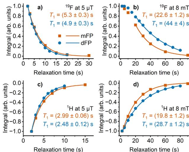
Fig. 8 Relaxation time analysis of SABRE-hyperpolarised  $^{19}\text{F}$  and  $^1\text{H}$  nuclei at selected magnetic fields.  $^{19}\text{F}$  at (a) 5  $\mu\text{T}$  and (b) 8 mT.  $^1\text{H}$  at (c) 5  $\mu\text{T}$  and (d) 8 mT.
