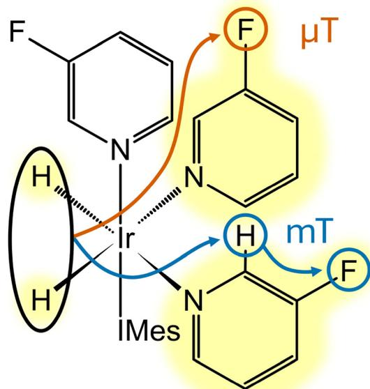
Fig. 2 Upon activation, the iridium catalyst forms a hexacoordinate complex in which the spin order transfer from parahydrogen to the ligands takes place.<sup>4</sup> The 14-spin system, with hydride protons and mFP ligands highlighted in yellow, was used in the spin dynamics simulations. Proposed polarisation transfer pathways are demonstrated in the  $\mu\text{T}$  (orange) and mT (blue) field-strength regimes.
