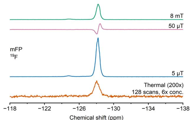
**Fig. 4** Comparison of  $^{19}\text{F}$  spectra from thermally polarised and SABRE-hyperpolarised mFP. The concentration of the thermally polarised sample is 6 times higher. The small peak seen at  $-124.8$  ppm corresponds to the mFP ligand bound in the equatorial position of the complex.
