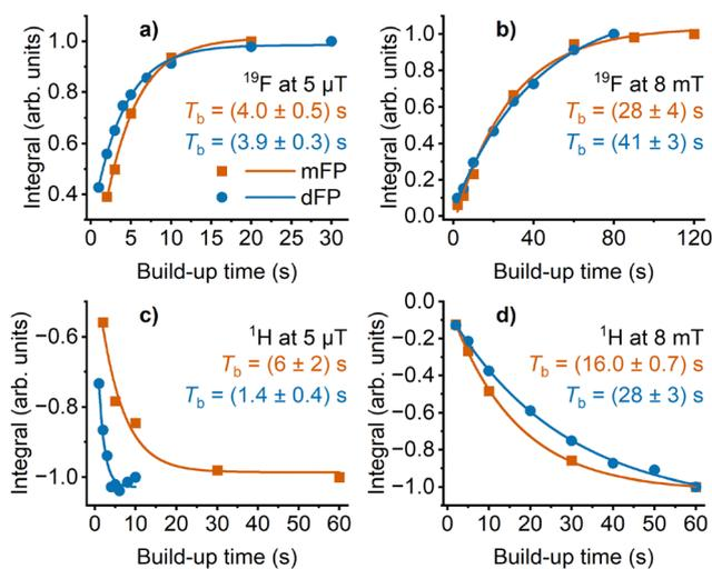
**Fig. 9** Determination of SABRE hyperpolarisation build-up times for  $^{19}\text{F}$  and  $^1\text{H}$  nuclei in mFP and dFP at different magnetic fields.  $^{19}\text{F}$  at (a) 5  $\mu\text{T}$  and (b) 8 mT.  $^1\text{H}$  at (c) 5  $\mu\text{T}$  and (d) 8 mT.
