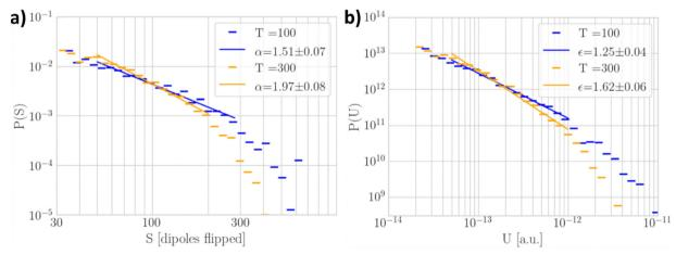
Fig. 5 Probability distribution of (a) event size and (b) energy for the same system settings at a lower (T = 100 K) and higher (T = 300 K) temperature. The simulation parameters here were f = 1 kHz,  $n_x = n_y = 4$ ,  $n_z = 300$ , N = 10,  $\sigma_N = 1$ .
