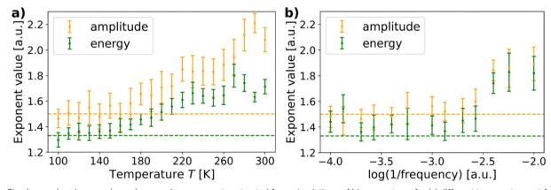
Fig. 6 Size (orange) and energy (green) power-law exponents extracted from simulations of bigger systems for (a) different temperatures at f = 1 KHz and (b) sweeping frequencies at T = 160 °C. The horizontal lines indicate the values calculated from the mean field plasticity model. The simulation parameters here were  $n_x = n_y = 4$ ,  $n_z = 300$ , N = 10,  $\sigma_N = 1$
