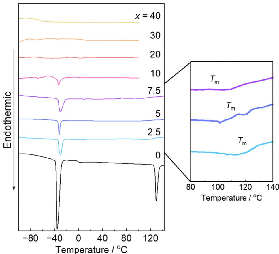
Fig. 2 DSC profiles of [C<sub>2</sub>epyr]Mg- $x$ . The figure on the right shows the DSC profiles near the melting point of [C<sub>2</sub>epyr]Mg- $x$  ( $x = 2.5, 5, 7.5$ ).
