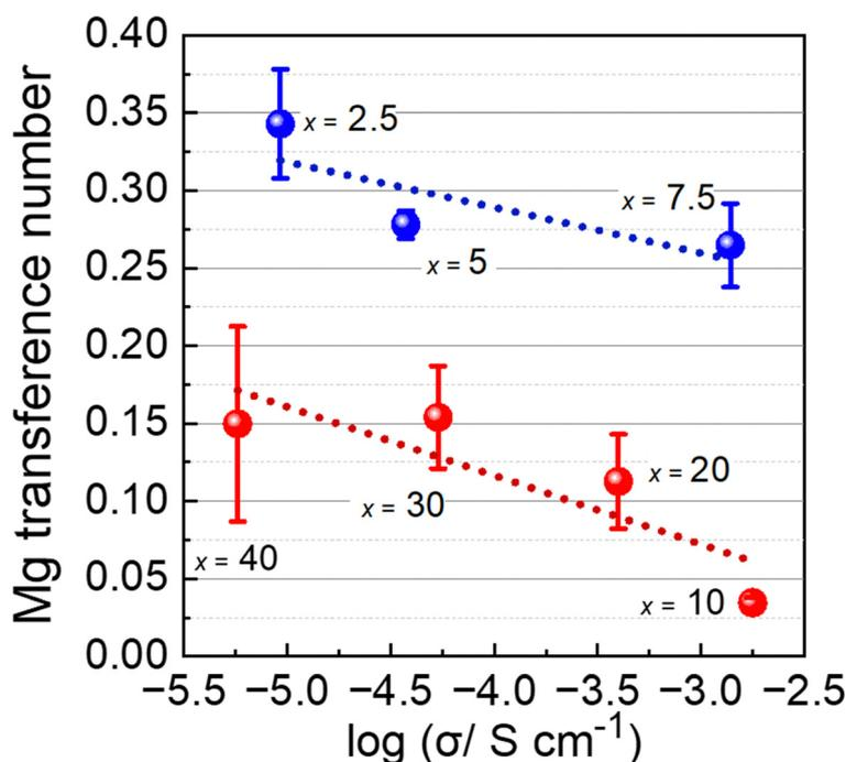
Fig. 6 Relationship between the Mg-ion transference number and ionic conductivity of  $[\text{C}_2\text{epyr}]\text{Mg}-x$  at 25 °C (blue: solid, red: liquid, error bars represent standard deviations from the mean).
