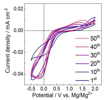
Fig. 7 Cyclic voltammograms of [C₂epyr]Mg-5 at 60 °C.
