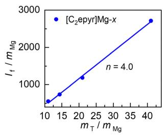
Fig. 3 Plots of  $I_{\rm f}/m_{\rm Mg}$  versus  $m_{\rm T}/m_{\rm Mg}$  for the 1220 cm $^{-1}$  band of [C2epyr]Mg-x. n: solvation number.
