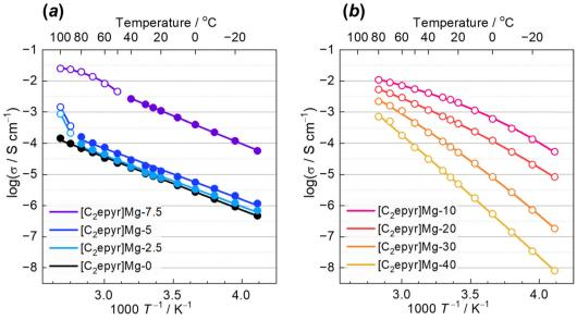
Fig. 5 Arrhenius plots of ionic conductivity for [C<sub>2</sub>epyr]Mg-x ((a) x = 0, 2.5, 5, 7.5 and (b) x = 10, 20, 30, 40). Open plots: liquid, closed plots: solid.
