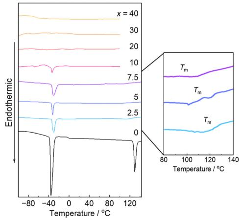
Fig. 2 DSC profiles of  $[C_2 \text{epyr}]Mg-x$ . The figure on the right shows the DSC profiles near the melting point of  $[C_2 \text{epyr}]Mg-x$  (x = 2.5, 5, 7.5).
