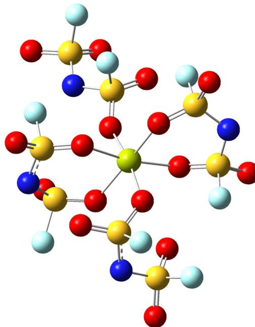
Fig. 4 Typical Mg<sup>2+</sup> solvation structure extracted from the snapshot. Light green: Mg, red: O, blue: N, yellow: S, light blue: F.
