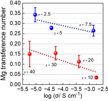
Fig. 6 Relationship between the Mg-ion transference number and ionic conductivity of [C2epyr]Mg-x at 25 °C (blue: solid, red: liquid, error bars represent standard deviations from the mean)
