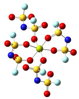
Fig. 4 Typical Mg<sup>2+</sup> solvation structure extracted from the snapshot. Light green: Mg, red: O, blue: N, yellow: S, light blue: F.
