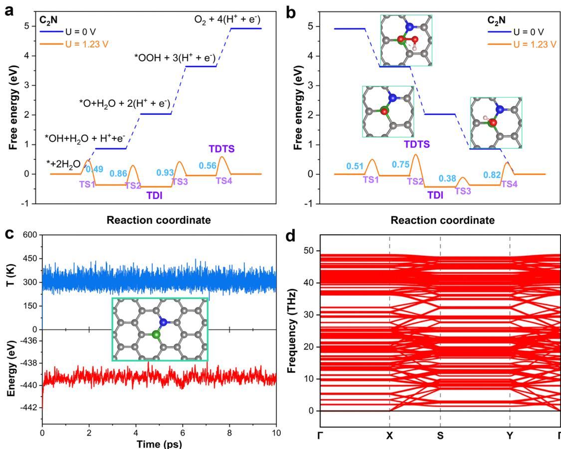
Fig. 3 OER (a) and ORR (b) free energy plots of the B-doped C<sub>2</sub>N substrate with four transition states. (c) Fluctuation of temperature and energy versus time (10 ps) in AIMD simulations. (d) Phonon dispersion spectra of the B-doped C<sub>2</sub>N potential structure.
