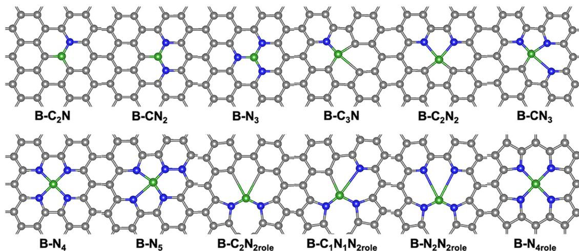
Fig. 1 Optimized models of single B-doped 2D graphene with different nitrogen species. Black, blue, and green represent C, N, and B, respectively.
