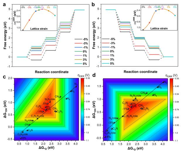
Fig. 4 Gibbs free energy plot of OER (a) and ORR (b) performance on the B-doped C2N structure with different strains. The inset images are the corresponding  $\eta^{ORR}$  and  $\eta^{ORR}$  versus strain curves. Contour images of  $\eta^{OER}$  (c) and  $\eta^{ORR}$  (d) as a function of  $\Delta E_{*OH}$  and  $\Delta E_{*O}$  constructed by the linear scaling relationship of B-N<sub>x</sub>-C structures
