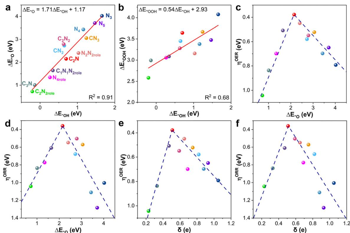
Fig. 2 Scaling relationships of intermediate adsorption energies for (a)  $^*O$  versus  $^*OH$  and (b)  $^*OOH$  versus  $^*OH$  on the twelve potential structures. Activity volcano plots of  $\eta^{OER}$  (c) and  $\eta^{ORR}$  (d) versus the free energies of  $^*O$  ( $\Delta E_{^*O}$ ). Volcano plots of  $\eta^{OER}$  (e) and  $\eta^{ORR}$  (f) as a function of the Bader charge ( $\delta$ , in units of e) of a single boron atom.
