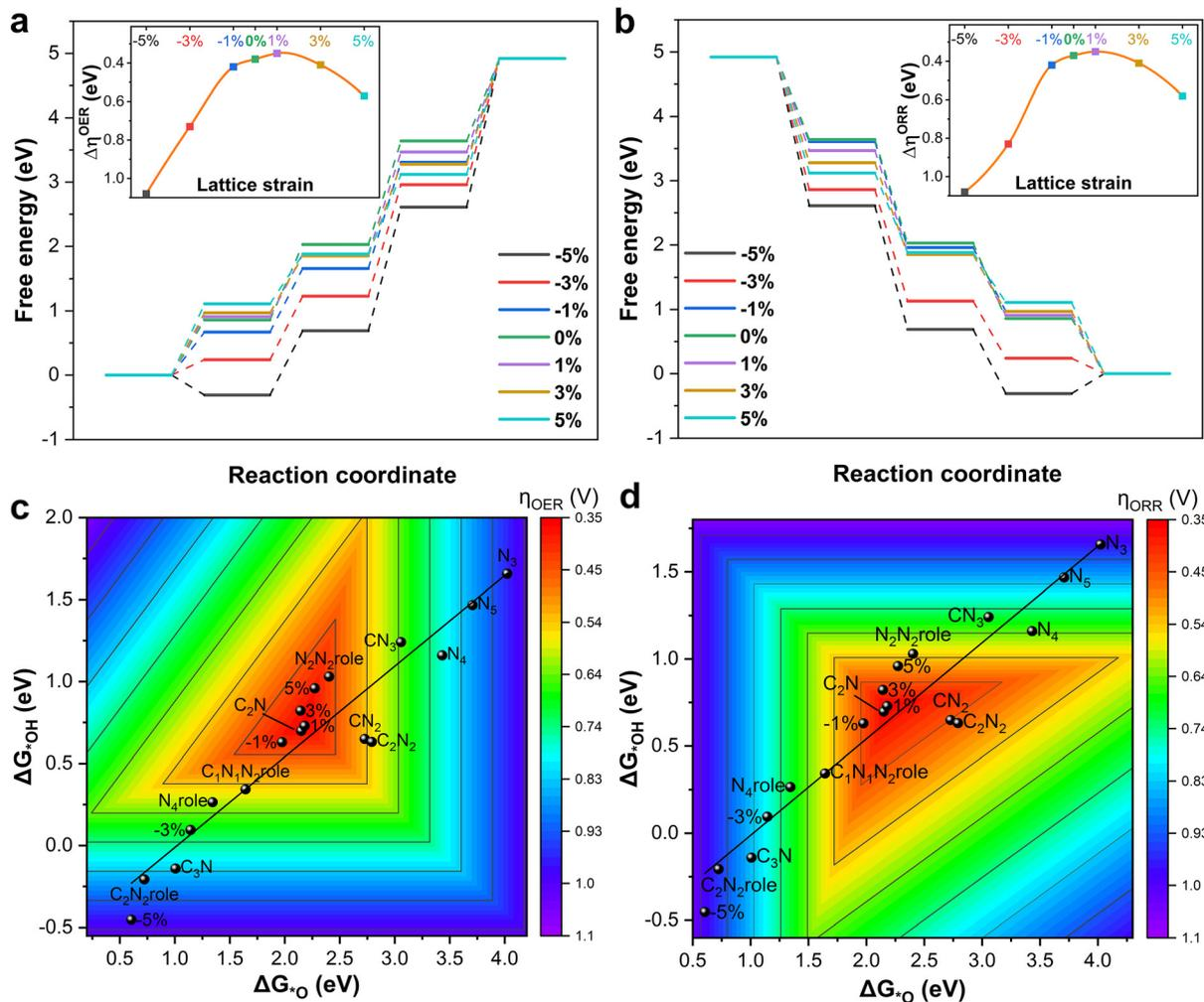
Fig. 4 Gibbs free energy plot of OER (a) and ORR (b) performance on the B-doped  $C_2N$  structure with different strains. The inset images are the corresponding  $\eta_{OER}^{ORR}$  and  $\eta_{ORR}^{ORR}$  versus strain curves. Contour images of  $\eta_{OER}^{ORR}$  (c) and  $\eta_{ORR}^{ORR}$  (d) as a function of  $\Delta E_{OH}$  and  $\Delta E_{+O}$  constructed by the linear scaling relationship of B- $N_x$ -C structures.
