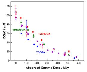
Fig. 5 DGA concentrations as a function of absorbed gamma dose in n-dodecane: TODGA ( $\blacksquare$ ), T2EHDGA ( $\bullet$ ), and DMDODGA ( $\blacktriangle$ ) from this work. Previously reported values for: TODGA (), 32 TODGA (), 12 and corrected for the electron density difference between Fricke and n-dodecane (1.04).
