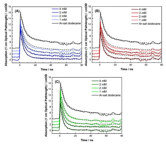
Fig. 3 Kinetic traces at 1600 nm for the interaction between the e<sub>solv</sub> and 1, 2, 3, and 4 mM (A) TODGA (-), (B) T2EHDGA (-), and (C) DMDODGA (-) in n-dodecane at 20.0 °C. Traces were offset by 1 mOD to aid in visibility of the reaction kinetics. Fits with eqn (5) are shown by the dashed lines (- -).
