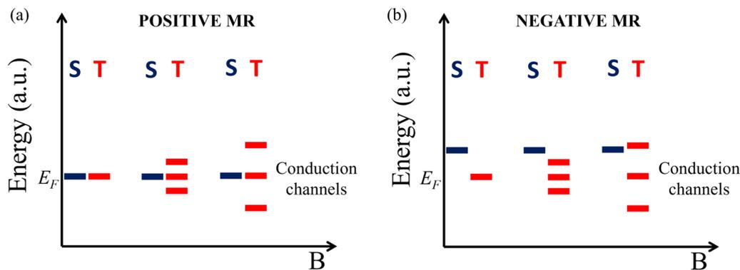
Fig. 5 The scheme of the MR mechanism for the (a) positive MR and (b) negative MR based on S–T states.<sup>14</sup> Due to exchange energy, the elevated initial T states in (b) created more conduction channels as the magnetic field was applied.
