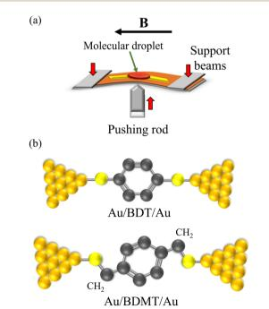
Fig. 1 Illustration of (a) MCBJ setup and (b) single-molecule junctions of BDT and BDMT molecules. For simplicity, the hydrogen (H) atoms were omitted in the figure. In Au/BDMT/Au junctions, the phenyl ring and Au/S interfaces are separated by a methylene (-CH<sub>2</sub>) unit.
