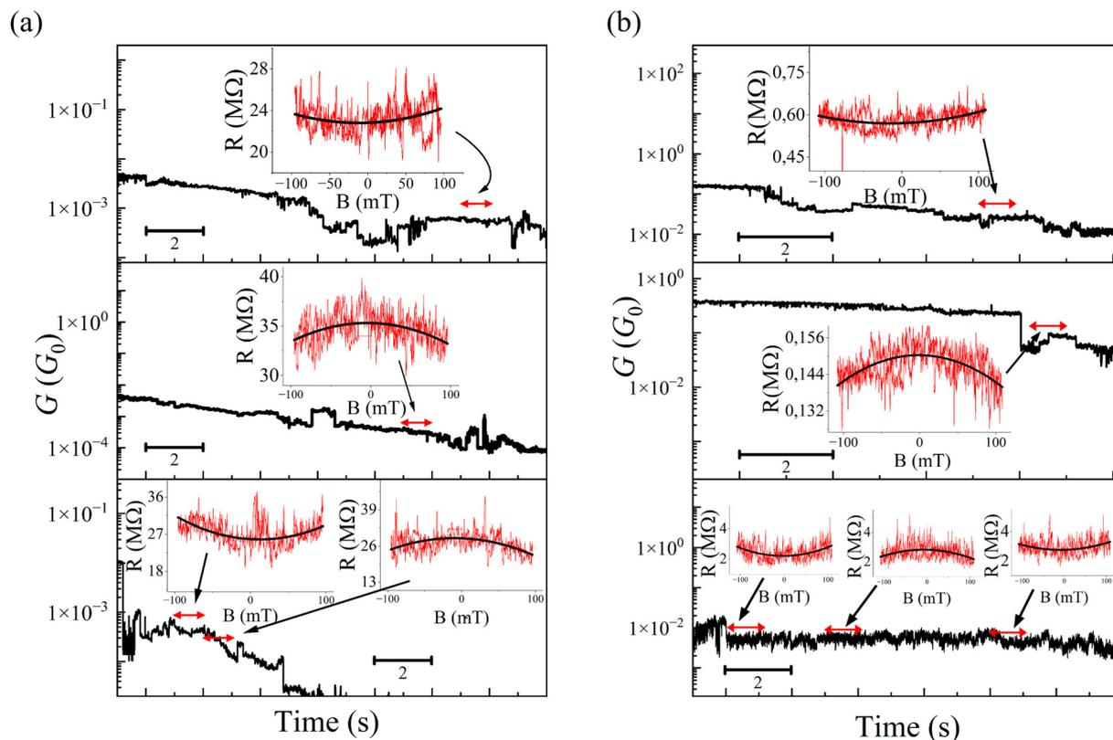
Fig. 3 Various individual  $G$ -traces for (a) Au/BDT/Au and (b) Au/BDMT/Au junctions, with the MR curves fitted by a parabolic function shown in the insets. Red arrows indicate the periods of the MR measurements. Scale bars represent the time scale, in seconds, during the breaking process.
