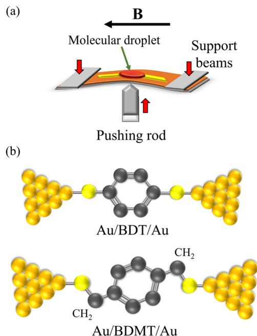
**Fig. 1** Illustration of (a) MCBJ setup and (b) single-molecule junctions of BDT and BDMT molecules. For simplicity, the hydrogen (H) atoms were omitted in the figure. In Au/BDMT/Au junctions, the phenyl ring and Au/S interfaces are separated by a methylene ( $-\text{CH}_2$ ) unit.
