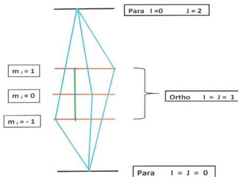
**Fig. 5** Hydrogen conversion and nuclear magnetic resonance lines. The magnetic resonance lines in green are compared to the ortho–para lines in blue. The ortho manifold is amplified in comparison to the two neighboring para energies.
