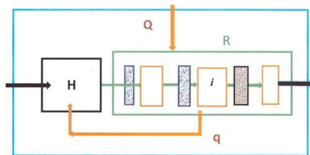
Fig. 9 Retroaction scheme in DOV storage vessels.  $\text{LH}_2$  is loaded in  $H$ . Part  $q$  (in brown) of the entering heat flux ( $Q$  in brown) reaches the reservoir  $H$  inducing a directional hydrogen current (in black) that crosses the microporous catalysis (in grey) and is directed towards the fuel cell. By reversing the arrows, the flows in the liquefiers can be schematically represented.
