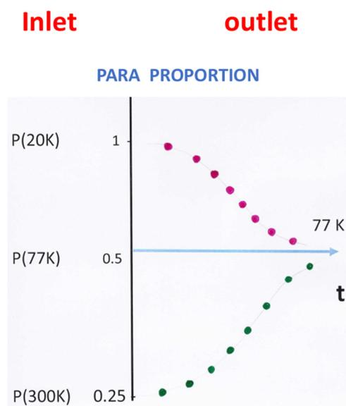
Fig. 7 Para proportion in a hydrogen flow. The para proportion of a hydrogen flow is represented as a function of the residence time  $t$  the hydrogen spends in the reactive conversion cell (arbitrary units are a function of pressure). Inlet proportions correspond to the experimental conditions (catalyst at 77 K).
