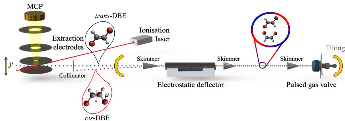
Fig. 1 Schematic of the molecular-beam setup used for the electrostatic spatial separation and investigation of the photoionisation and photofragmentation of *cis*- and *trans*-1,2-dibromoethene ( $C_2H_2Br_2$ , DBE) with a femtosecond (fs) laser at a wavelength of 775 nm.
