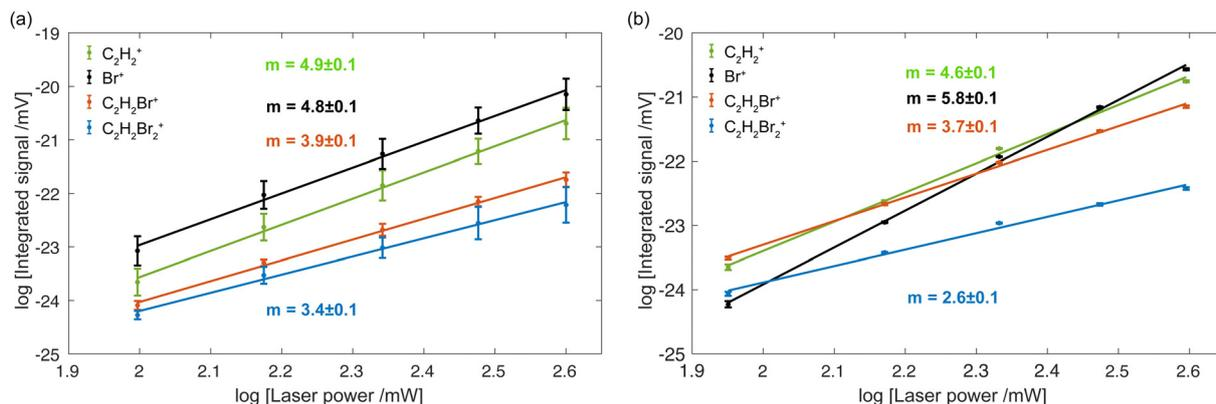
Fig. 5 Doubly logarithmic representation of ion yields vs. fs-laser power for (a) an isomeric mixture of DBE and (b) *cis*-DBE. The straight lines are linear fits to the data with  $m$  denoting the slope. Uncertainties represent the standard deviations of the fits. Each data point represents the average of three measurements with each being an average over 2000 laser shots.
