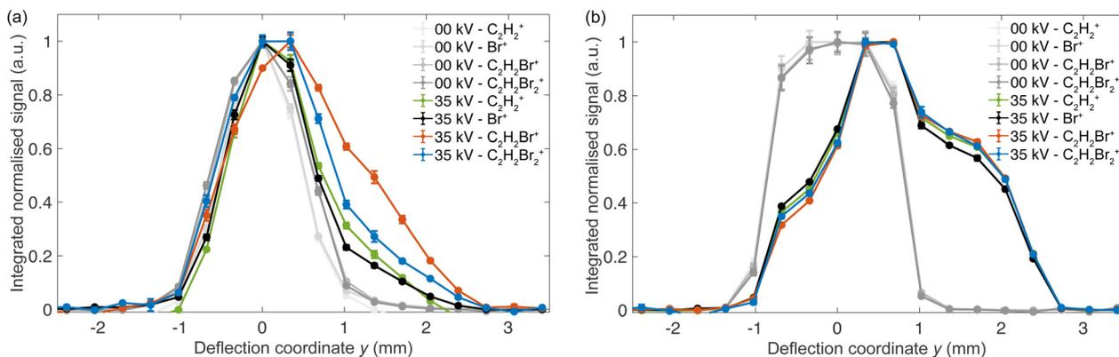
Fig. 3 Deflection profiles of the parent and fragments of (a) a  $\approx 1:1$  mixture of the DBE isomers and (b) *cis*-DBE obtained by fs-laser ionisation. All profiles have been normalised with respect to their maxima. Error bars represent the standard error of three measurements with each being an average over 2000 laser shots.
