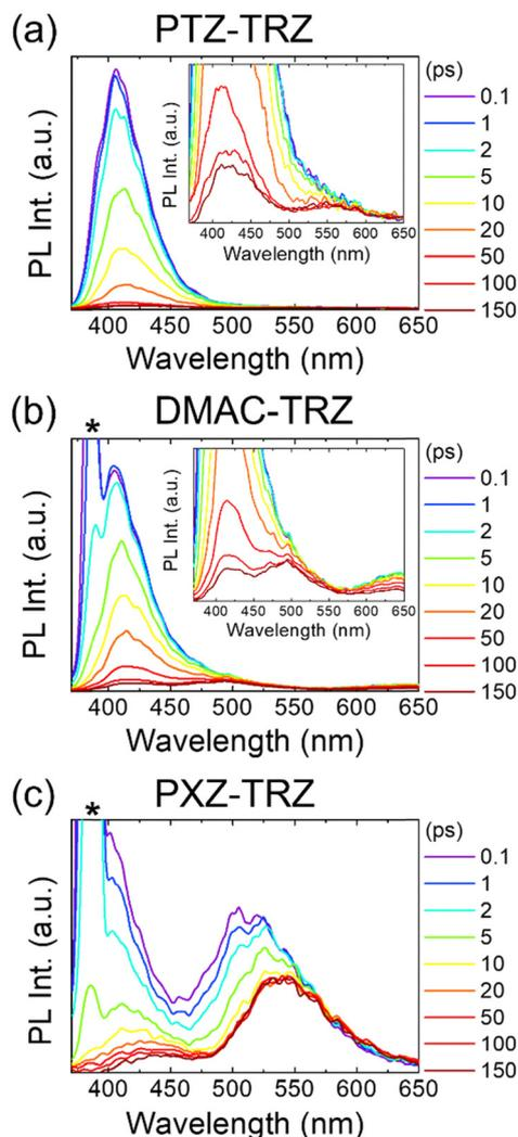
Fig. 3 The TR-PL spectra on the picosecond timescale of (a) **PTZ-TRZ**, (b) **DMAC-TRZ**, and (c) **PXZ-TRZ** in toluene solution. Insets of (a) and (b) show the enlarged TR-PL spectra in the range of 375–650 nm. The asterisk represents the Raman scattering signal.
