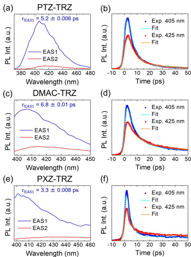
Fig. 4 The results of a global analysis of the TR-PL spectra. The evolution associated spectra (EAS) of (a) **PTZ-TRZ**, (c) **DMAC-TRZ**, and (e) **PXZ-TRZ**. Comparison of the time profiles at 405 and 425 nm of the TR-PL spectra to the fitting of a global analysis in (b) **PTZ-TRZ**, (d) **DMAC-TRZ**, and (f) **PXZ-TRZ**. We used a sequential two-state model for all the molecules.
