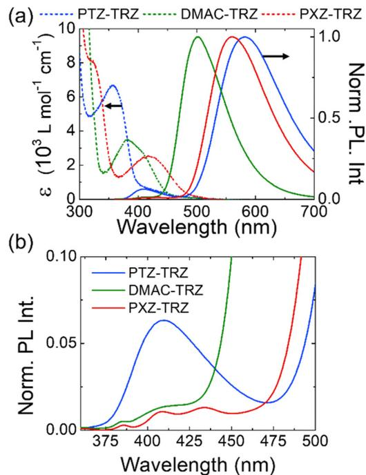
Fig. 2 (a) The UV-vis absorption spectra (dashed lines) and the normalized PL spectra (solid lines) of **PTZ-TRZ** (blue), **DMAC-TRZ** (green), and **PXZ-TRZ** (red) in toluene solution. The concentration of the solutions for PL measurements is 0.1 mM. (b) Expanded normalized steady-state PL spectra in the range of 360–500 nm.
